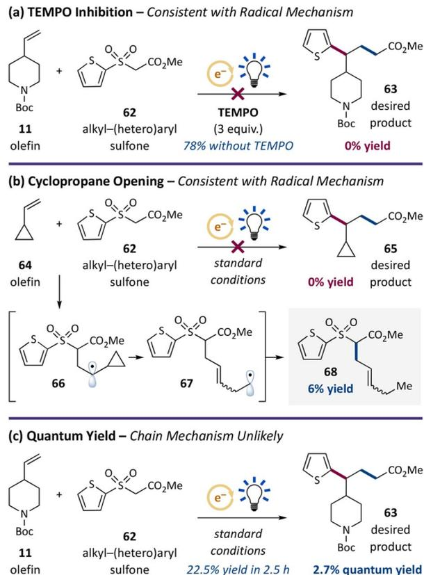
**Scheme 2** Preliminary mechanistic experiments were consistent with the proposed radical mechanism (Fig. 2). (a) Addition of a persistent radical TEMPO completely inhibited the reaction. (b) Using vinylcyclopropane (**64**) as the olefin afforded only ring-opened byproduct **68** and none of desired product **65**. (c) A low quantum yield (2.7%) was measured, which disfavors a chain mechanism. See ESI† for detailed procedures.
