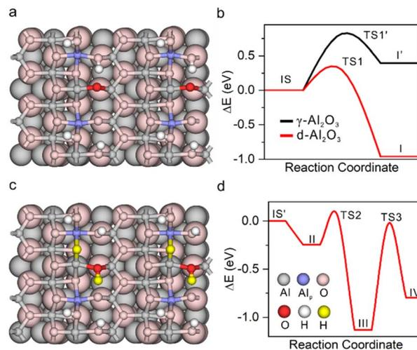
Fig. 3 Structure of (a) d-Al<sub>2</sub>O<sub>3</sub> and (c) d-Al<sub>2</sub>O<sub>3</sub> with heterolytically dissociated H<sub>2</sub>. The colour code is shown in panel (d). Energetic profiles of (b) H<sub>2</sub> activation over  $\gamma$ -Al<sub>2</sub>O<sub>3</sub> and d-Al<sub>2</sub>O<sub>3</sub>, and (d) following stepwise hydrogenation of C<sub>2</sub>H<sub>4</sub> over d-Al<sub>2</sub>O<sub>3</sub>.
