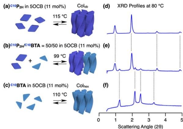
Fig. 7 (a–c) Schematic representations of the formation of columnar LC and (d–f) XRD profiles at 80 °C of (a and d)  $C^{10}P_{2H}$ , (b and e)  $C^{10}P_{2H}/C^{10}BTA = 50/50$  in 5OCB (11 mol%) and (c and f)  $C^{10}BTA$  in 5OCB (11 mol%). The temperatures shown above the arrows in (a–c) are the LC phase transition temperatures obtained by DSC on cooling ( $5\text{ °C min}^{-1}$ ).
