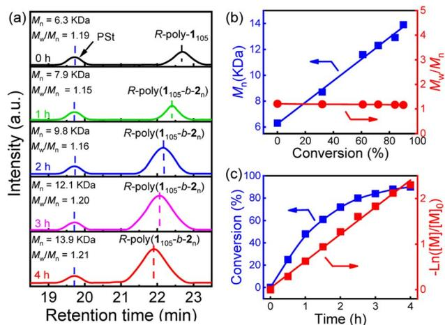
Fig. 2 (a) Time-dependent SEC for the copolymerization of 2 catalyzed by Pd(II)-terminated R-poly-1<sub>105</sub>. (b) Plots of  $M_n$  and  $M_w/M_n$  of R-poly(1<sub>m</sub>-*b*-2<sub>n</sub>) vs. the conversion of 2. (c) Plots of conversion and  $-\ln([M]/[M]_0)$  values vs. the polymerization time.
