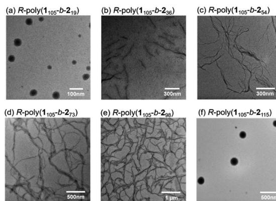
Fig. 6 TEM images of *R*-poly( $1_{105}$ -*b*-2<sub>19</sub>) (a), *R*-poly( $1_{105}$ -*b*-2<sub>36</sub>) (b), *R*-poly( $1_{105}$ -*b*-2<sub>54</sub>) (c), *R*-poly( $1_{105}$ -*b*-2<sub>73</sub>) (d), and *R*-poly( $1_{105}$ -*b*-2<sub>98</sub>) (e), and *R*-poly( $1_{105}$ -*b*-2<sub>115</sub>) (f).
