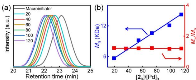
Fig. 1 (a) SEC curves for the copolymerization of **2** initiated by *R*-poly-**1<sub>105</sub>** carrying the Pd(II)-terminus at different **2**-to-Pd(II) ratios. (b) Plots of  $M_n$  and  $M_w/M_n$  of *R*-poly(**1<sub>m</sub>-b-2<sub>n</sub>**)s vs. the **2**-to-Pd(II) ratios.
