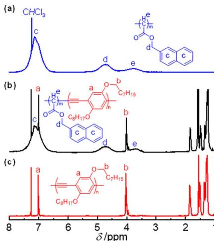
Fig. 3  $^1\text{H}$  NMR ( $\text{CDCl}_3$ , 600 MHz) spectra of the polymers:  $R$ -poly- $1_{105}$  (a),  $R$ -poly( $1_{105}$ - $b$ - $2_{98}$ ) (b), and poly- $2_{30}$  (c) measured at room temperature.
