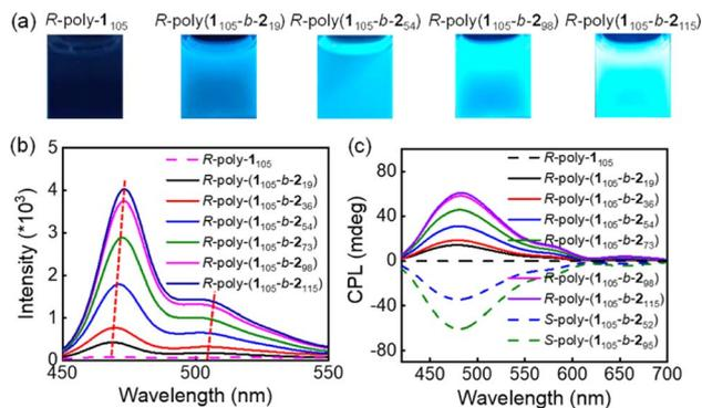
Fig. 7 (a) Photographs of poly( $1_{105}$ - $b$ - $2_n$ ) copolymers under UV light of 365 nm. (b) Emission spectra of poly( $1_{105}$ - $b$ - $2_n$ ) copolymers irradiated at 365 nm. (c) CPL spectra of poly( $1_{105}$ - $b$ - $2_n$ ) irradiated at 380 nm. The spectra were recorded in THF at 25 °C with  $c = 0.2$  mg mL<sup>-1</sup>.
