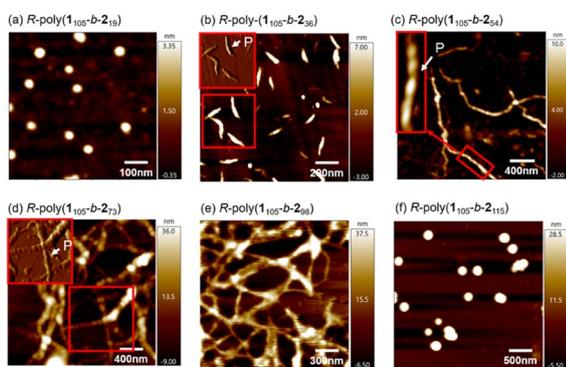
Fig. 5 AFM images of *R*-poly( $1_{105}$ -*b*-2<sub>19</sub>) (a), *R*-poly( $1_{105}$ -*b*-2<sub>36</sub>) (b), *R*-poly( $1_{105}$ -*b*-2<sub>54</sub>) (c), *R*-poly( $1_{105}$ -*b*-2<sub>73</sub>) (d), and *R*-poly( $1_{105}$ -*b*-2<sub>98</sub>) (e), and *R*-poly( $1_{105}$ -*b*-2<sub>115</sub>) (f).
