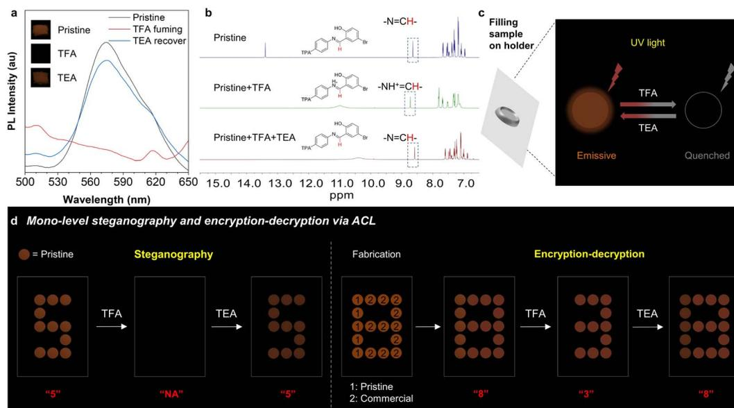
Fig. 5 (a) PL spectra of *p*-TPA-Br as solid: pristine, sample fumed with TFA, sample fumed with TEA. Inset: fluorescence photographs taken after different treatments. (b)  $^1\text{H}$  NMR spectra of *p*-TPA-Br in  $\text{CDCl}_3$  before and after TFA and TEA in 7.0–15.0 ppm region. (c) Schematic diagram of the sample holder with TFA and TEA responses. (d) Schematic diagram of mono-level steganography and encryption-decryption.
