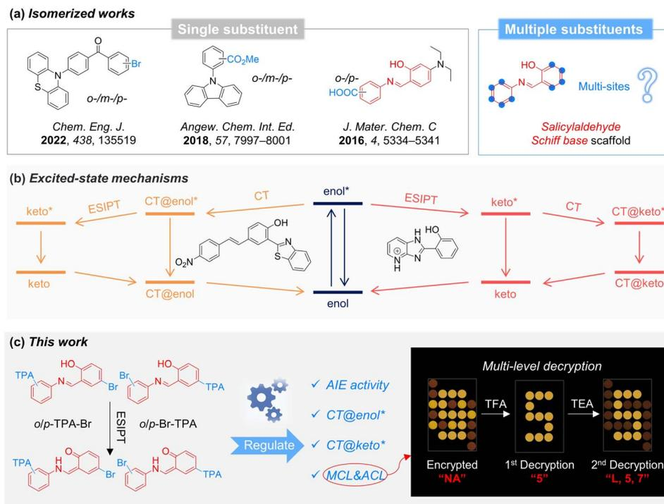
**Fig. 1** (a) Structures of conventional single-substituent molecules (I–III) and the salicylaldehyde Schiff base scaffold with multi-site substitutions (IV). (b) The different paths and order of excited-state processes of CT and ESIPT. (c) Molecular design and properties of multi-substituted salicylaldehyde Schiff bases in this work. CT: charge transfer, ESIPT: excited-state intramolecular proton transfer, MCL: mechanochromic luminescence, ACL: acidichromic luminescence.
