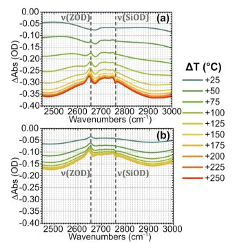
Fig. 3 FTIR temperature ramp difference spectra of ZSM-5 in flowing HOD/H $_2$ O vapour on heating relative to 100 °C (a) and 175 °C (b) at the indicated  $\Delta T$  values. The corresponding difference spectra relative to other temperatures are shown in the ESI, Section 4.† The location of  $\nu$ (SiOD) silanol modes and  $\nu$ (ZOD) Brønsted acid modes are highlighted.
