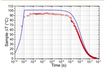
Fig. 8 Average sample temperature across the probed region vs. time for a temperature jump from 175 °C  $T_{Act}$  as determined experimentally (red) and from simulations (blue). The simulation uses the best estimates for input parameters
