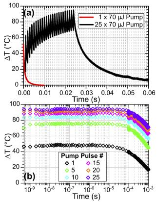
Fig. 11 (a) Sample temperature evolution for HOD/H $_2$ O in ZSM-5 at  $T_{\rm Init}=125$  °C following pumping by 1× (red) and 25× (black) 70  $\mu$ J pump pulses. (b) Comparison of temperature evolution in first 1 ms following indicated pulse number in 25-pulse burst showing nanosecond time resolution throughout full range.
