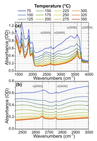
Fig. 2 IR absorption (FTIR) spectra from 1400–4000 cm $^{-1}$  of ZSM-5 held in flowing HOD/H<sub>2</sub>O vapour at indicated temperatures showing (a) all features and (b) the detection range used in the time-resolved spectroscopy. The location of  $\nu$ (SiOH) silanol modes, free  $\nu$ (ZOH) Brønsted acid modes and their deuterated equivalents are highlighted.
