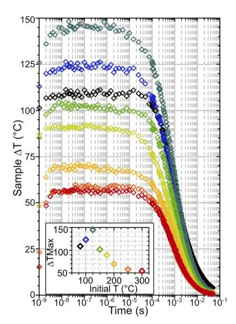
Fig. 6 Sample heating vs. time after ns laser heating for  $HOD/H_2O$  dosed ZSM-5 at different initial temperatures calculated based on changes in silanol mode intensity. The inset plot shows the maximum  $\Delta T$  achieved against initial temperature. The colour scheme of the heating transients corresponds to that in the inset.
