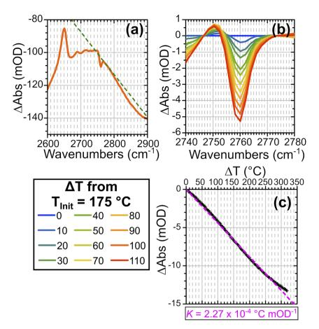
Fig. 5 (a) FTIR difference spectrum of  $\Delta T = 50$  °C from  $T_{\text{Init}} = 175$  °C showing a linear baseline fit to isolate silanol mode contributions. (b) Comparison of the  $\nu$ (SiOD) feature in baseline subtracted difference spectra at indicated  $\Delta T$  values showing increase in intensity of negative feature with increased  $\Delta T$ . (c) Variation of  $\nu$ (SiOD) negative intensity with  $\Delta T$  showing linear relationship with slope 1/K.
