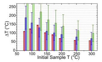
Fig. 9 Average temperature jump measured between  $10^{-8}$  and  $10^{-5}$  s as determined by: experiment based on changes in silanol mode intensity (red); heat transfer simulations (blue); energy absorption calculations (green). Frror bars for simulation and calculation values are based on the uncertainties in the input parameters.
