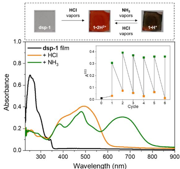
Fig. 9 Top: glass substrate spin-coated with **dsp-1** and exposed to ammonia and then hydrochloric acid vapours. Bottom: electronic absorption spectra of the thin film before and after exposure to vapours. Inset: reversibility of pH-switching monitored at 660 nm.
