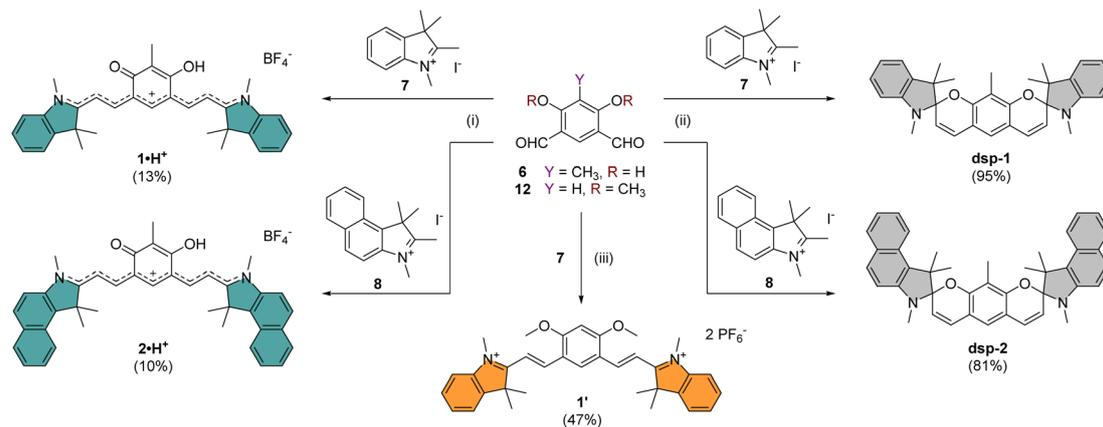
**Scheme 1** Synthesis of chromophores **1** and **2** under their cationic or neutral forms. Conditions: (i) **6**, EtOH, piperidine, 95 °C, 16 h, then aq. HBF<sub>4</sub>, 25 °C; (ii) **6**, EtOH, piperidine, 95 °C, 16 h, then aq. NaHCO<sub>3</sub>; (iii) **12**, Ac<sub>2</sub>O, AcONa, 100 °C, 16 h, then aq. KPF<sub>6</sub>.
