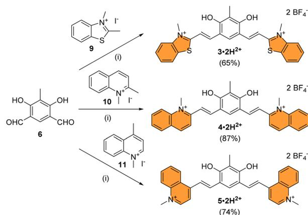
**Scheme 2** Synthesis of chromophores **3–5** under their dicationic forms. Conditions: (i) EtOH, piperidine, 95 °C, 16 h, then aq. HBF<sub>4</sub>, 25 °C, 5 min to 5 h.
