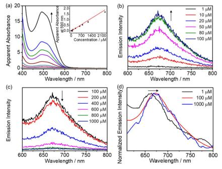
Fig. 5 (a) Electronic absorption spectra of  $\bf 6$  in aqueous solutions at various concentrations (from 5.73 to 2319  $\mu$ M). Inset: the plot of absorbance at 590 nm against concentration. Emission spectra of  $\bf 6$  in water at various concentrations from (b) 1 to 100  $\mu$ M and (c) 100 to 1000  $\mu$ M. (d) Normalized emission spectra of  $\bf 6$  in water at concentrations of 1  $\mu$ M, 100  $\mu$ M and 1000  $\mu$ M.
