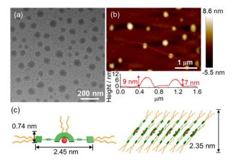
Fig. 6 (a) TEM and (b) AFM images prepared from a solution of  $\bf 6$  in water ([Pt] =  $2.0 \times 10^{-4}$  M). (c) Schematic diagram of the proposed lamellar structure of  $\bf 6$  in water.
