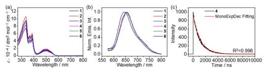
Fig. 2 (a) Electronic absorption spectra and (b) normalized emission spectra of 1-6 in degassed DMSO solutions ( $10^{-5}$  M) at 298 K. (c) The monoexponential phosphorescence decay trace (detected at the emission band maxima) of 4 in the degassed DMSO solution at 298 K.
