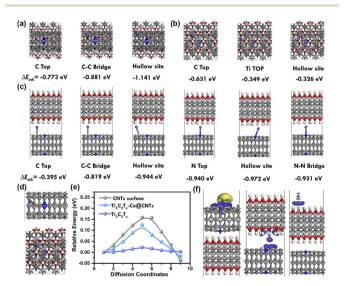
Fig. 5 Theoretical simulations of potassium adsorption/diffusion on the heterointerface between NCNTs and  $Ti_3C_2T_x$ . Potassium adsorption on the surface of (a) NCNTs, (b)  $Ti_3C_2T_x$ , and (c)  $Ti_3C_2T_x$ -Co@NCNTs, (d) potassium diffusion paths on the  $Ti_3C_2T_x$ -Co@NCNTs, (e) the corresponding diffusion barrier energy, and (f) the electron density differences.
