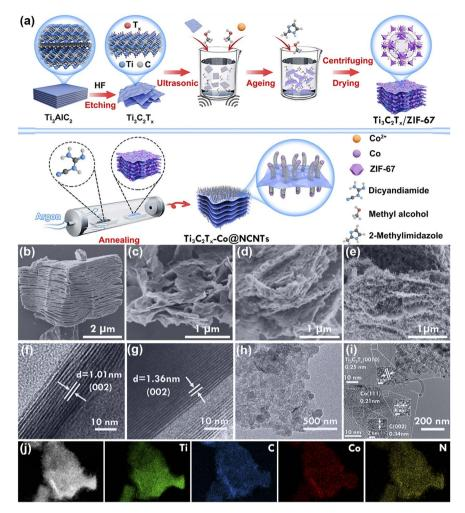
Fig. 1 (a) Scheme for the synthesis route of  $Ti_3C_2T_x$ -Co@NCNTs. SEM images of (b)  $Ti_3C_2T_x$ , (c) the exfoliated  $Ti_3C_2T_x$ , (d)  $Ti_3C_2T_x$ /ZIF-67, and (e)  $Ti_3C_2T_x$ -Co@NCNTs, TEM images of (f)  $Ti_3C_2T_x$ , (g)  $Ti_3C_2T_x$ , (h)  $Ti_3C_2T_x$ /ZIF-67, and (i)  $Ti_3C_2T_x$ -Co@NCNTs and (j) elemental mapping of  $Ti_3C_2T_x$ -Co@NCNTs.
