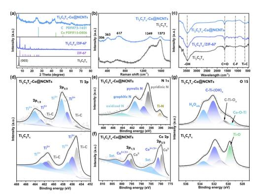
Fig. 2 (a) XRD patterns of  $Ti_3C_2T_x$ ,  $Ti_3C_2T_x$ /ZIF-67, and  $Ti_3C_2T_x$ -Co@NCNTs, (b) Raman spectrum of  $Ti_3C_2T_x$ , and  $Ti_3C_2T_x$ -Co@NCNTs, (c) FT-IR spectrum of  $Ti_3C_2T_x$ ,  $Ti_3C_2T_x$ /ZIF-67 and  $Ti_3C_2T_x$ -Co@NCNTs, and high-resolution XPS spectra of (d)  $Ti_3C_2T_x$  (e) N 1s, (f) Co 2p, and (g) O 1s.
