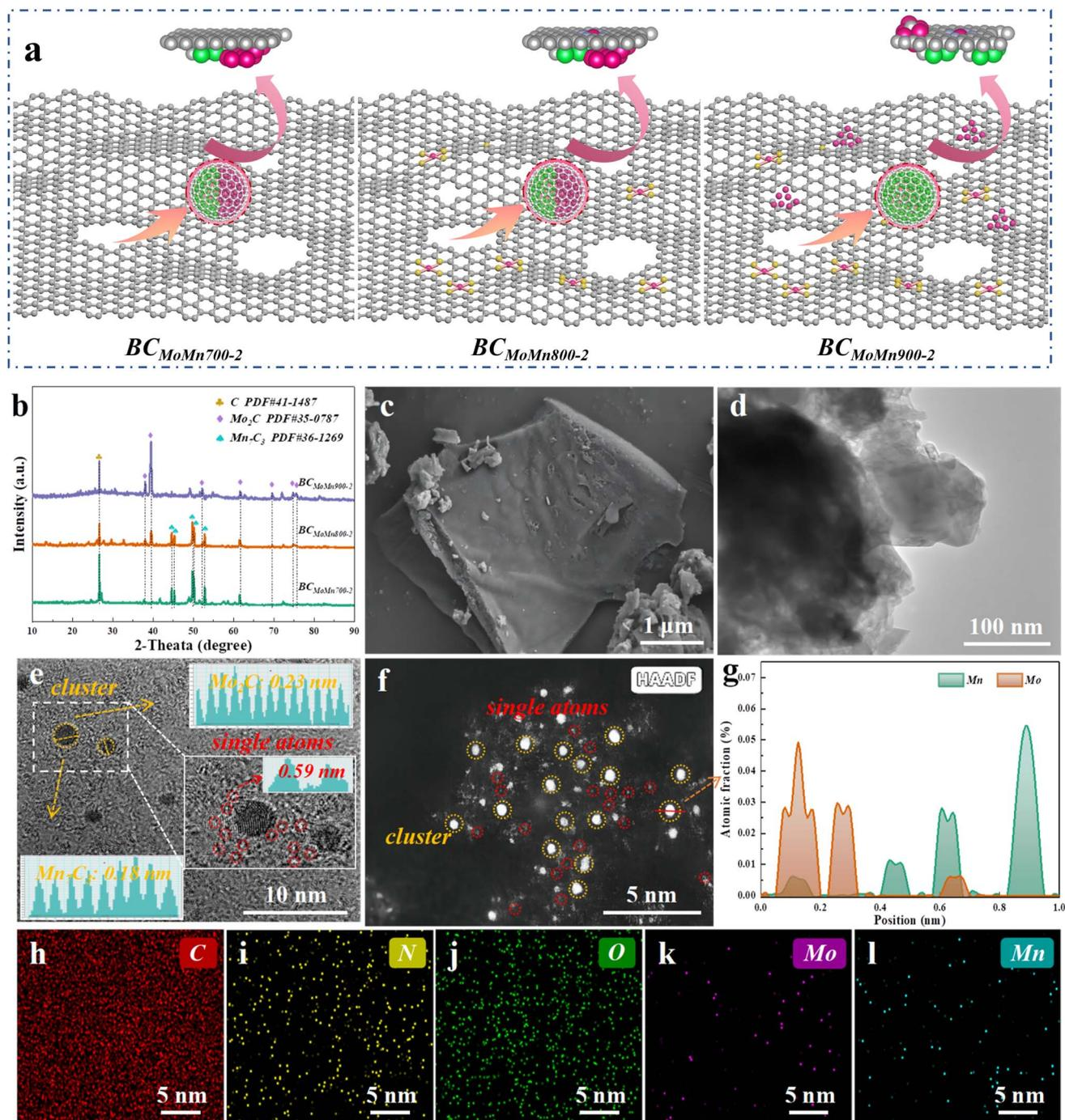
Fig. 1 Catalyst synthesis and structural characterization. (a) Schematic illustration of catalyst structure evolution at different preparation temperatures. (b) XRD spectra of  $BC_{MoMn700-2}$ ,  $BC_{MoMn800-2}$ , and  $BC_{MoMn900-2}$ . (c) FESEM, (d) TEM, (e) HRTEM, (f) dark-field HAADF-STEM, (g) corresponding EDS line-scan elemental of  $BC_{MoMn800-2}$ , and (h–l) EDS mappings of  $BC_{MoMn800-2}$ .
