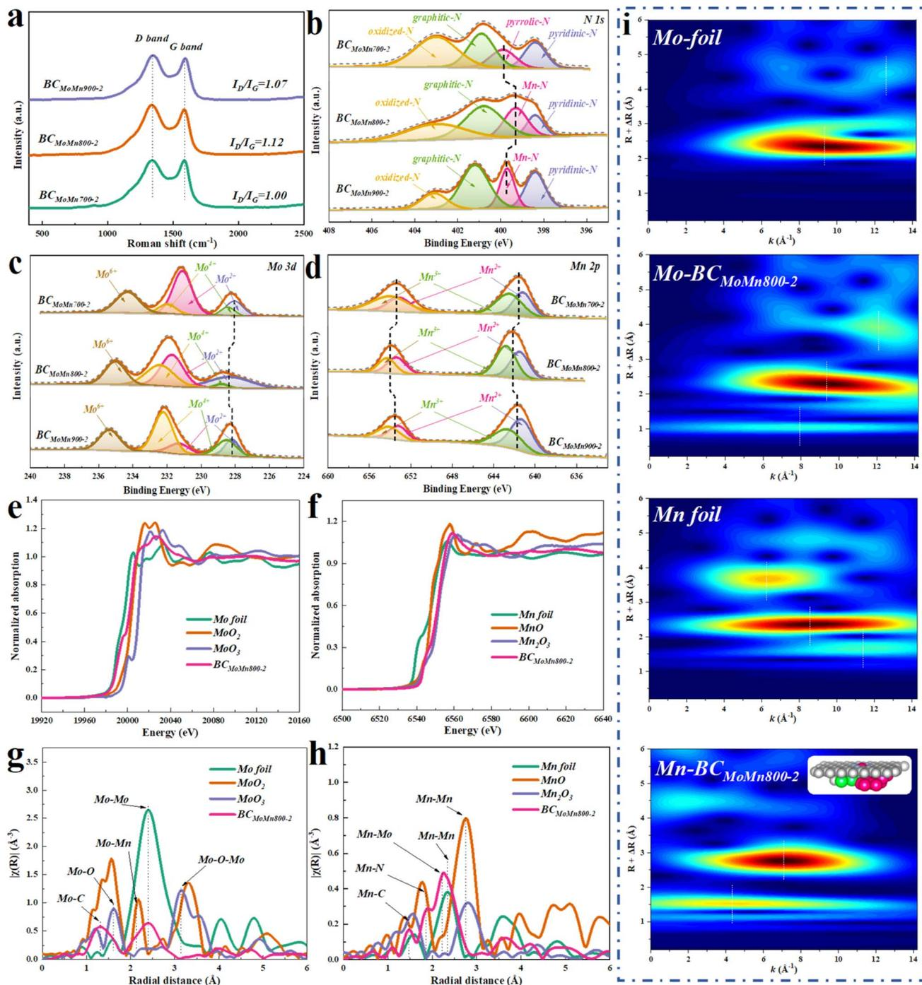
Fig. 2 Chemical composition characterization. The (a) Raman, (b) high-resolution Mo 2p, (c) Mn 2p, and (d) N 1s spectra of  $BC_{MoMn700-2}$ ,  $BC_{MoMn800-2}$ , and  $BC_{MoMn900-2}$ . (e, g) Mo and (f, h) Mn K-edge XANES and Fourier transforms of the EXAFS spectra of  $BC_{MoMn800-2}$ . (i) Wavelet transforms for the  $k^3$ -weighted EXAFS signals of Mo foil, Mn foil, and  $BC_{MoMn800-2}$ .
