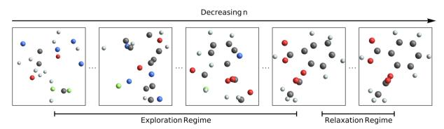
Fig. 1 Schematic showing the diffusion process for a molecule over the course of *n* steps. For high *n* (left panel), the atomic species and positions are extremely random. At test time, the model predicts progressively less noisy molecules until arriving at a final prediction (right panel).
