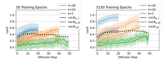
Fig. 6 QM9 model/force comparison. Left: cosine of the angles between the sum of the next k steps predicted by diffusion  $(\Delta_k)$ , the DFT-computed forces (f), and the path directly from the current geometry to the DFT-computed ground state (gs). Curves are averaged across atoms from 45 molecules from the QM9 validation set. Shaded regions represent one standard deviation above and below the mean (the shaded region can exceed 1.0 because the distribution is not Gaussian).
