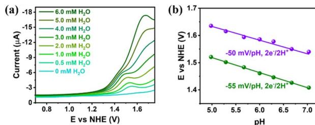
Fig. 4 (a) DPVs of  $\text{Gd}_6\text{Cu}_{24}\text{-AC}$  (0.25 mM) in  $\text{CH}_3\text{CN}$  with  $\text{Et}_4\text{NClO}_4$  (0.1 M) before and after addition of different amounts of  $\text{H}_2\text{O}$ . (b) Pourbaix diagram of  $\text{Gd}_6\text{Cu}_{24}\text{-AC}$  (0.25 mM) in NaAc/HAc (0.5 M, pH 4.98–7.03) buffer solution.  $E_p$  values are cited rather than  $E_{1/2}$  due to chemical irreversibility.
