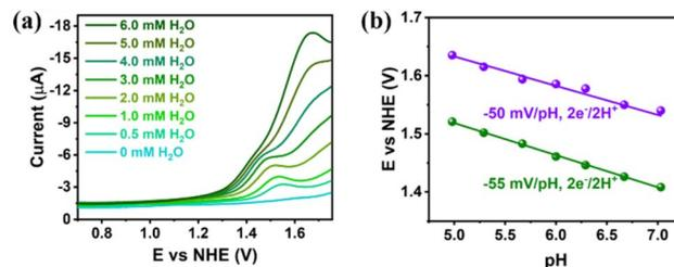
Fig. 4 (a) DPVs of  $\text{Gd}_6\text{Cu}_{24}\text{-AC}$  (0.25 mM) in  $\text{CH}_3\text{CN}$  with  $\text{Et}_4\text{NClO}_4$  (0.1 M) before and after addition of different amounts of  $\text{H}_2\text{O}$ . (b) Pourbaix diagram of  $\text{Gd}_6\text{Cu}_{24}\text{-AC}$  (0.25 mM) in NaAc/HAc (0.5 M, pH 4.98–7.03) buffer solution.  $E_p$  values are cited rather than  $E_{1/2}$  due to chemical irreversibility.
