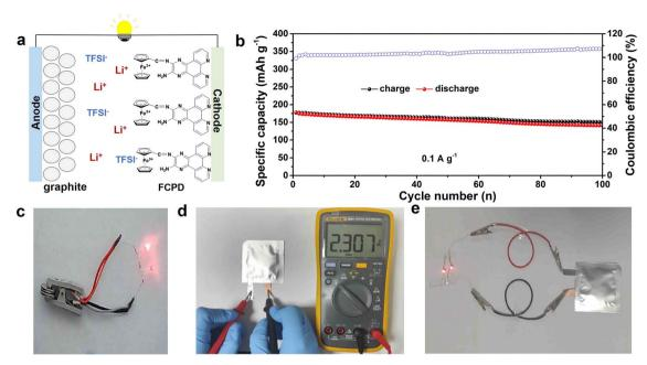
Fig. 6 (a) Schematic diagram of the graphite//FCPD full cell. (b) Cycling performance of the graphite//FCPD full cell at  $0.1 \text{ A g}^{-1}$ . (c) The digital photo of the full cell lighting diodes. (d) and (e) Practical evaluation of the graphite//FCPD pouch battery.
