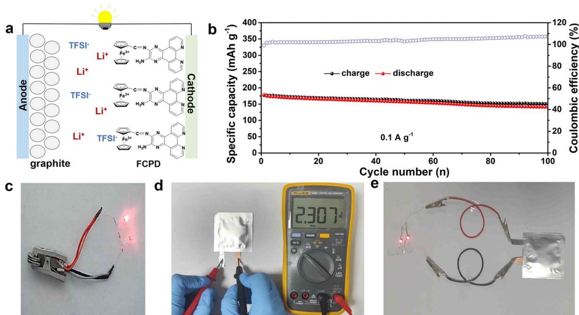
Fig. 6 (a) Schematic diagram of the graphite//FCPD full cell. (b) Cycling performance of the graphite//FCPD full cell at  $0.1 \text{ A g}^{-1}$ . (c) The digital photo of the full cell lighting diodes. (d) and (e) Practical evaluation of the graphite//FCPD pouch battery.
