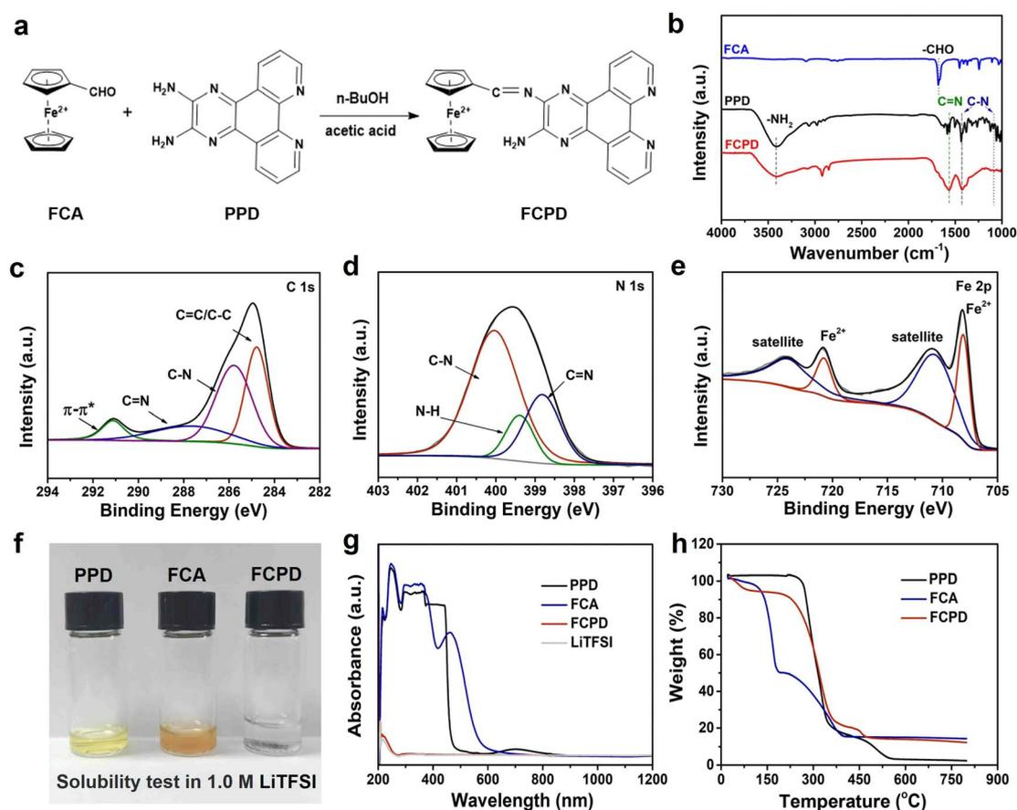
Fig. 1 (a) Schematic synthesis of the FCPD cathode. (b) FT-IR spectra of PPD, FCA, and FCPD. (c)–(e) High-resolution XPS spectra of C 1s, N 1s, and Fe 2p for FCPD. (f) Photographs of PPD, FCA, and FCPD soaked in an electrolyte (1 M LiTFSI in DME/DOL), respectively. (g) UV-vis spectra of the electrolyte (1 M LiTFSI in DME/DOL) and the electrolytes after soaking PPD, FCA, and FCPD. (h) Thermogravimetric analysis of PPD, FCA, and FCPD.
