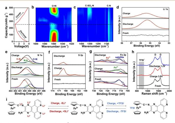
Fig. 5 (a) The 2nd charge/discharge profiles at 0.05 A  $g^{-1}$  and (b) and (c) corresponding in situ FT-IR contour map of the FCPD cathode. (d)–(g) High-resolution XPS spectra of Li 1s, N 1s, S 2p, and Fe 2p of the FCPD cathode at different charge/discharge states. (h) Ex situ Raman spectra of the FCPD cathode at different charge/discharge states. (i) Proposed dual ion storage mechanisms for the FCPD cathode.
