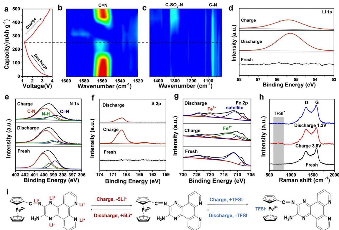
Fig. 5 (a) The 2nd charge/discharge profiles at  $0.05 \text{ A g}^{-1}$  and (b) and (c) corresponding *in situ* FT-IR contour map of the FCPD cathode. (d)–(g) High-resolution XPS spectra of Li 1s, N 1s, S 2p, and Fe 2p of the FCPD cathode at different charge/discharge states. (h) *Ex situ* Raman spectra of the FCPD cathode at different charge/discharge states. (i) Proposed dual ion storage mechanisms for the FCPD cathode.
