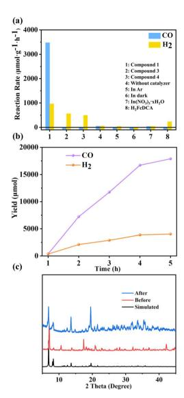
Fig. 7 (a) Reaction rates under different conditions; (b) photocatalytic performance test chart of compound 1; (c) powder XRD patterns for compound 1 before and after photocatalytic reaction.
