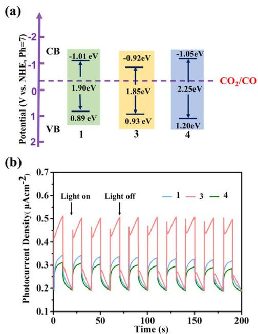
Fig. 6 (a) Energy-level diagram of 1, 3 and 4; (b) 0.4 V-bias photocurrent responses of electrodes derived for 1, 3 and 4 in 0.2 M Na<sub>2</sub>SO<sub>4</sub> aqueous solution under repetitive chopped visible light irradiation.
