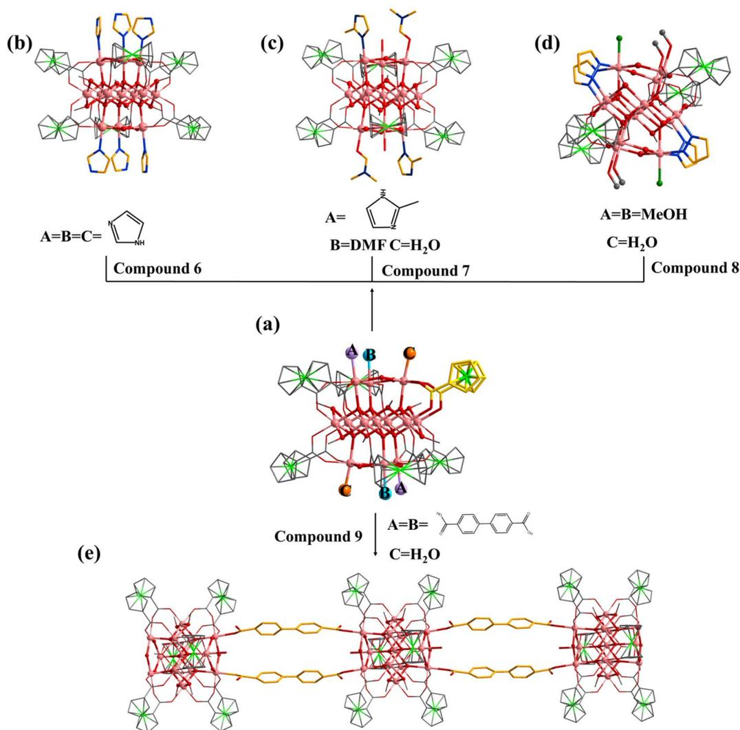
Fig. 5 (a)  $[In_{13}]$  as a secondary building unit; (b) compound 6 ( $A = B = C = HIm$ ); (c) compound 7 ( $A = 2\text{-mim}$ ,  $B = DMF$ ,  $C = H_2O$ ); (d) compound 8 ( $A = B = MeOH$ ,  $C = H_2O$ ); (e) compound 9 ( $A = B = BPDC$ ,  $C = H_2O$ ). A, B and C represent different substitution sites.
