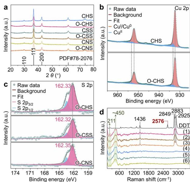
**Fig. 2** Structural characterizations. (a) XRD patterns of CHS, O-CHS, CSS, O-CSS, CNS, and O-CNS. (b) High-resolution Cu 2p XPS spectra of CHS and O-CHS. (c) High-resolution S 2p XPS spectra of O-CHS, O-CSS, and O-CNS. (d) Raman spectra of DDT, O-CHS (1), O-CSS (2), O-CNS (3), CHS (4), CSS (5), and CNS (6).
