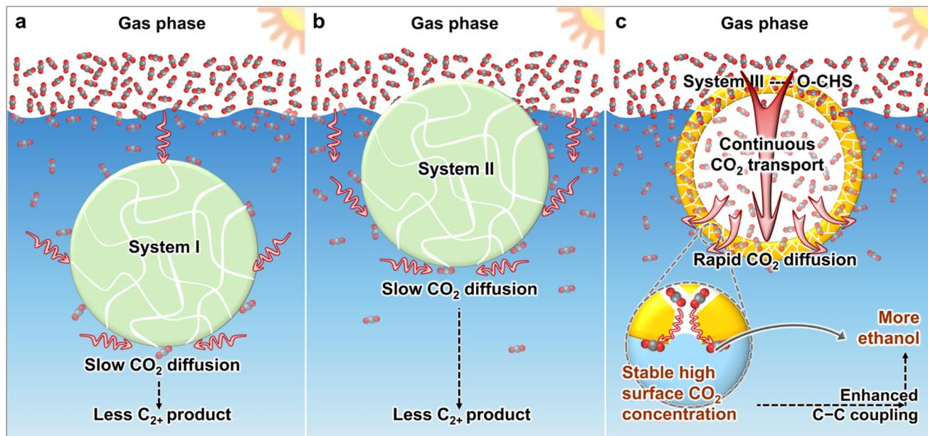
**Scheme 1** Schematics of  $\text{CO}_2$  diffusion in systems involving reported hydrophobic materials and the designed O-CHS. (a) System I with hydrophobic materials suspended in the aqueous solution. (b) System II with hydrophobic materials floating on the aqueous solution. (c) System III with the designed O-CHS. The gas phase of  $\text{CO}_2$  is depicted in white, and the aqueous solution is depicted in blue. The gray and red balls represent C and O atoms, respectively.
