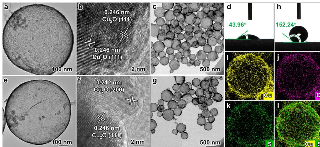
**Fig. 1** Morphologies and wettability of CHS and O-CHS. (a and c) TEM images of CHS. (b) HRTEM image of CHS. (d) WCA of CHS. (e and g) TEM images of O-CHS. (f) HRTEM image of O-CHS. (h) WCA of O-CHS. (i–k) EDS mapping images of Cu, O, and S for O-CHS, respectively. (l) Overlapping EDS mapping signals of Cu and S for O-CHS.
