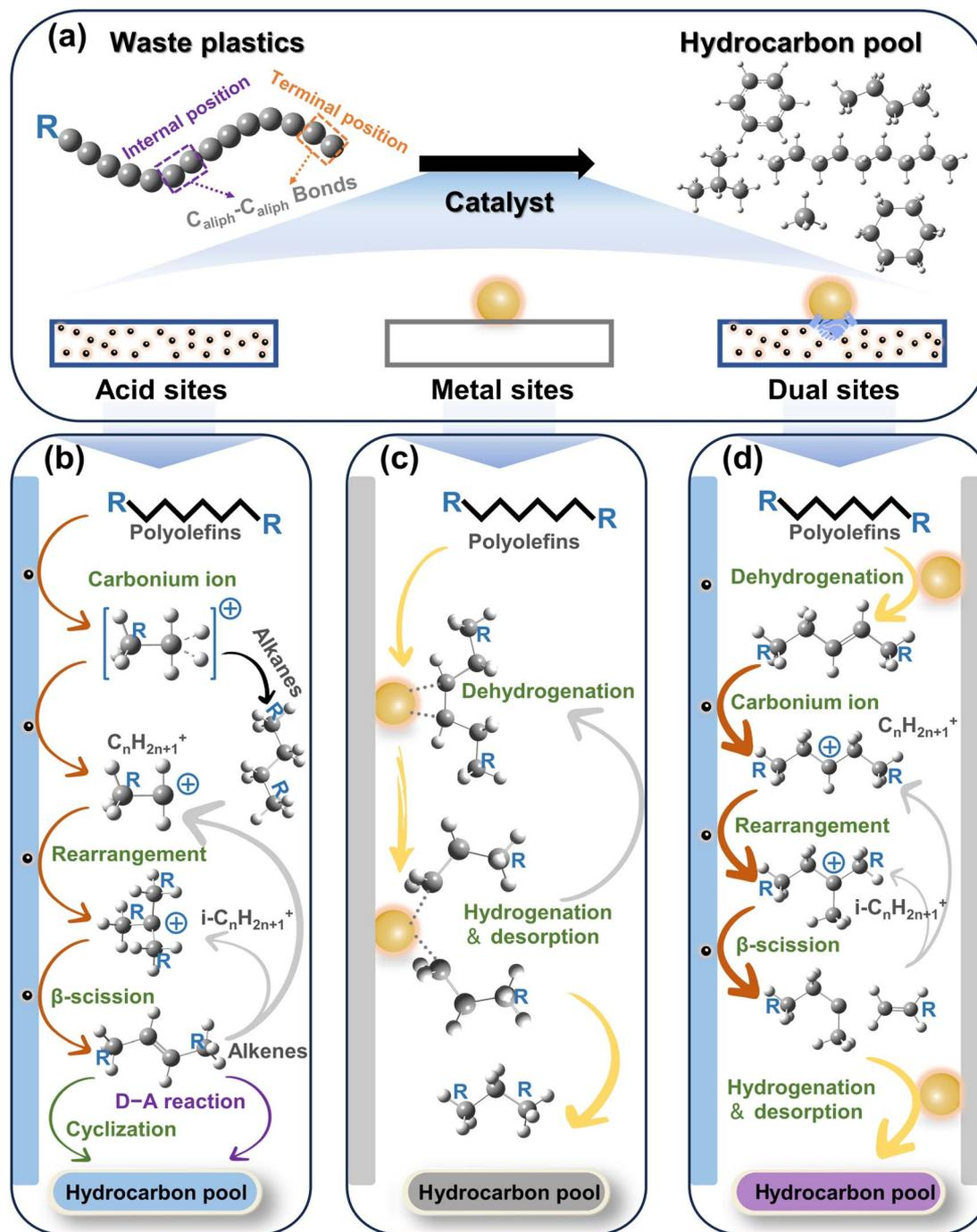
Fig. 2 (a) Schematic illustration of the upcycling of polyolefins via C<sub>aliph</sub>-C<sub>aliph</sub> bond activation. (b-d) Schematic diagrams of the upgradation of polyolefins when C<sub>aliph</sub>-C<sub>aliph</sub> bonds are activated over (b) the acid sites, (c) the metal sites, and (d) the dual sites.
