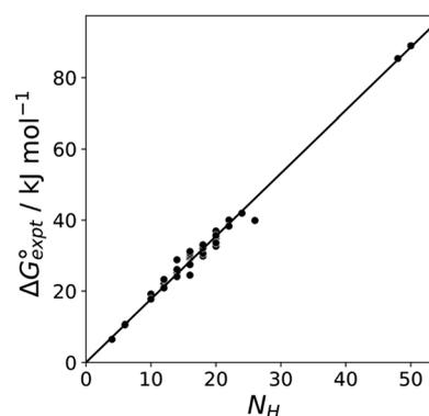
Fig. 11 Experimental free energy of transfer of alkanes from  $n$ -hexadecane to water ( $\Delta G_{\text{expt}}^{\circ}$ ) plotted as a function of the number of hydrogen atoms ( $N_H$ ).
