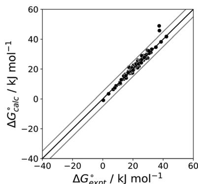
Fig. 13 Comparison of the experimental free energy of transfer of 108 unsaturated hydrocarbons from *n*-hexadecane to water ( $\Delta G_{\text{expt}}^{\circ}$ ) with the value calculated using the AIP model in SSIMPLE ( $\Delta G_{\text{calc}}^{\circ}$ ). The black line is  $y = x$ , and the grey lines indicate deviations of  $\pm 5$  kJ mol<sup>-1</sup> (RMSE = 1.8 kJ mol<sup>-1</sup>).
