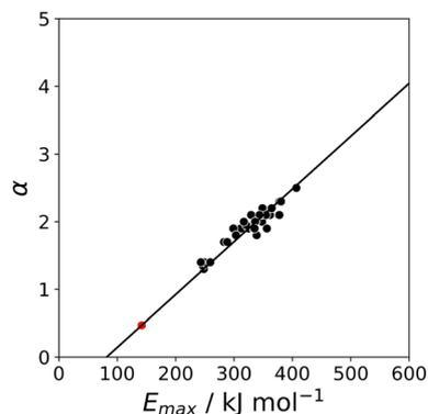
Fig. 12 Relationship between the experimentally measured H-bond parameter  $\alpha$  for non-polar donors and the value of  $E_{\max}$  calculated on the 0.0104 e bohr<sup>-3</sup> electron density isosurface using DFT (B3LYP/6-31G\* or B3LYP/6-311G\*\* for bromine and iodine). The best fit straight line was constrained to pass through the alkane CH point shown in red ( $m_{\alpha} = 0.0078$  kJ<sup>-1</sup> mol,  $c_{\alpha} = -0.64$ ,  $r^2 = 0.93$ ).
