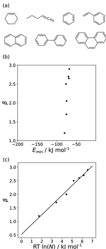
Fig. 7 (a) Structures of hydrocarbon  $\pi$ -systems with different numbers of carbon atoms in the  $\pi$ -system ( $N$ ). (b) Comparison of the experimentally measured H-bond parameter  $\beta$  for these compounds with the value of  $E_{\min}$  calculated on the 0.0020 e bohr $^{-3}$  electron density isosurface (DFT B3LYP/6-31G\*). (c) Comparison of  $\beta$  with  $N$ . The line is the best linear fit ( $\beta = 0.36 RT \ln N + 0.53$ ,  $r^2 = 0.98$ ).
