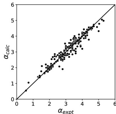
Fig. 3 Comparison of experimental  $\alpha$  parameters for H-bond donors and  $\sigma$ -holes ( $\alpha_{\text{expt}}$ ) with the corresponding values calculated with eqn (1) ( $\alpha_{\text{calc}}$ ) using  $m_\alpha$  and  $c_\alpha$  parameters from the lines of best fit in Fig. 1 (RMSE = 0.24).
