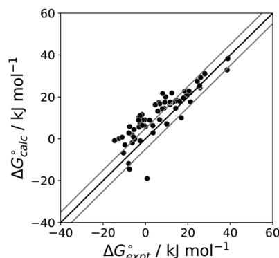
Fig. 14 Comparison of the experimental free energy of transfer of 65 compounds with positive  $\pi$ -systems from *n*-hexadecane to water ( $\Delta G_{\text{expt}}^{\circ}$ ) with the value calculated using the AIP model in SSIMPLE ( $\Delta G_{\text{calc}}^{\circ}$ ) ( $m_{\alpha} = 0.0206$  kJ<sup>-1</sup> mol,  $c_{\alpha} = 0.00$ , RMSE = 7.9 kJ mol<sup>-1</sup>). The black line is  $y = x$ , and the grey lines indicate deviations of  $\pm 5$  kJ mol<sup>-1</sup>.
