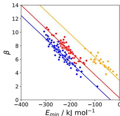
Fig. 4 Relationship between the experimentally measured H-bond parameter  $\beta$  and the value of  $E_{\text{min}}$  calculated on the 0.0300 e bohr<sup>-3</sup> electron density isosurface (DFT B3LYP/6-31G\*) for pyridine and imine nitrogen acceptors (blue,  $r^2 = 0.90$ ), amide oxygen acceptors (red,  $r^2 = 0.88$ ), and thionyl sulfur acceptors (yellow,  $r^2 = 0.70$ ). The lines are the best fit to eqn (3) with  $m_\beta = -0.0336$  kJ<sup>-1</sup> mol.
