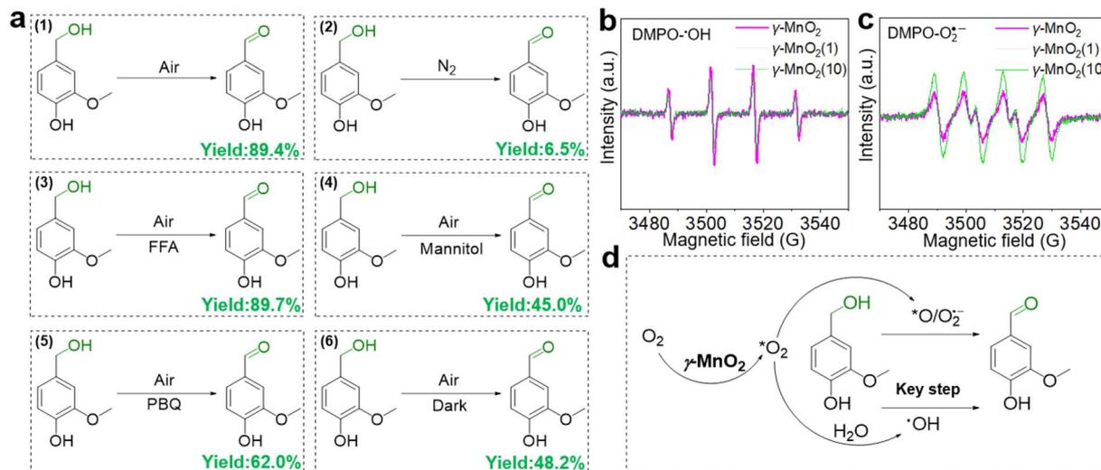
Fig. 4 Exploring the role of oxygen species in the oxidation of vanillyl alcohol over  $\gamma$ -MnO<sub>2</sub> catalyst. (a) Oxidation of vanillyl alcohol under different atmospheres or with various quenchers. (b and c) EPR spectra of DMPO-<sup>•</sup>OH and DMPO-O<sub>2</sub><sup>•-</sup> over various  $\gamma$ -MnO<sub>2</sub> catalysts. (d) Proposed the role of oxygen species in the oxidation of vanillyl alcohol. \*O<sub>2</sub> refers to the adsorbed oxygen.
