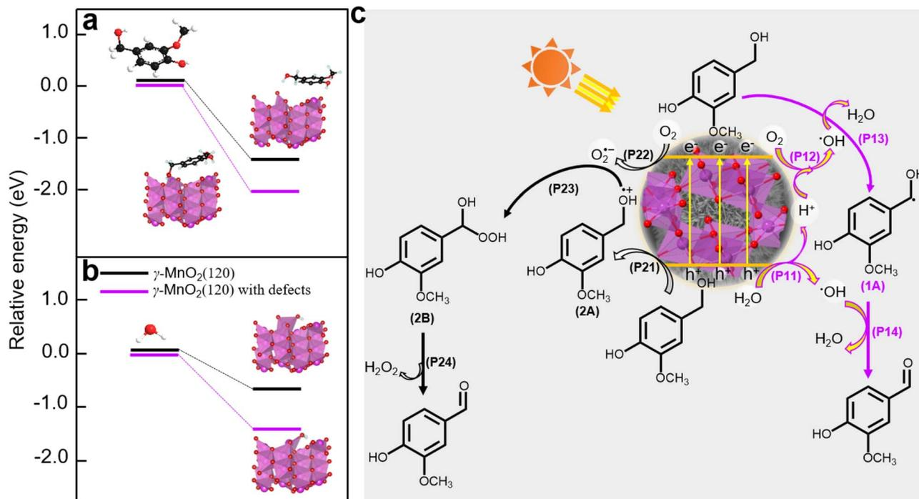
Fig. 6 (a) DFT calculations for vanillyl alcohol adsorbed on  $\gamma$ -MnO<sub>2</sub> catalyst with/without defects. (b) DFT calculations for H<sub>2</sub>O adsorbed on  $\gamma$ -MnO<sub>2</sub> catalyst with/without defects. (c) A plausible mechanism of oxidation of vanillyl alcohol to vanillin over  $\gamma$ -MnO<sub>2</sub> catalyst under air atmosphere.
