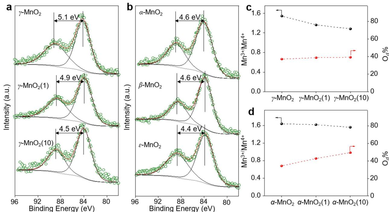
Fig. 2 Mn 3s XPS spectra for (a)  $\gamma$ -MnO<sub>2</sub> with different amounts of urea added in the synthesis and (b) MnO<sub>2</sub> with different crystal structures. The molar ratio of Mn<sup>3+</sup>/Mn<sup>4+</sup> and percentage of oxygen defects (O<sub>d</sub>) in different (c)  $\gamma$ -MnO<sub>2</sub> and (d)  $\alpha$ -MnO<sub>2</sub>.
