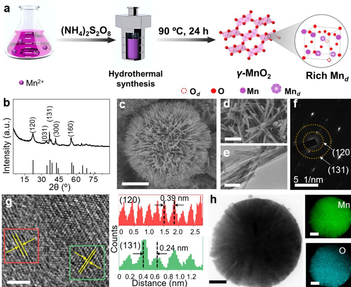
Fig. 1 (a) Schematic synthesis process of  $\gamma$ - $\text{MnO}_2$  catalysts with Mn defects ( $\text{Mn}_d$ ). (b) PXRD pattern, (c and d) SEM images, (e) TEM image, (f) SAED pattern, and (g) HRTEM image (left) and corresponding intensity plot (right) of  $\gamma$ - $\text{MnO}_2$  catalyst. (h) EDX elemental maps showing the distributions of Mn and O. Scale bars: (c) 2  $\mu\text{m}$ , (d) 500 nm, (e) 50 nm, (g) 2 nm, (h) 1  $\mu\text{m}$ .
