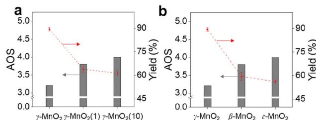
Fig. 3 Catalytic performance of  $\gamma$ -MnO<sub>2</sub> and comparison catalysts for oxidation of vanillyl alcohol to vanillin. (a) AOS-yield of vanillin on  $\gamma$ -MnO<sub>2</sub>, (b) AOS-yield of vanillin on MnO<sub>2</sub> with various crystal structures.
