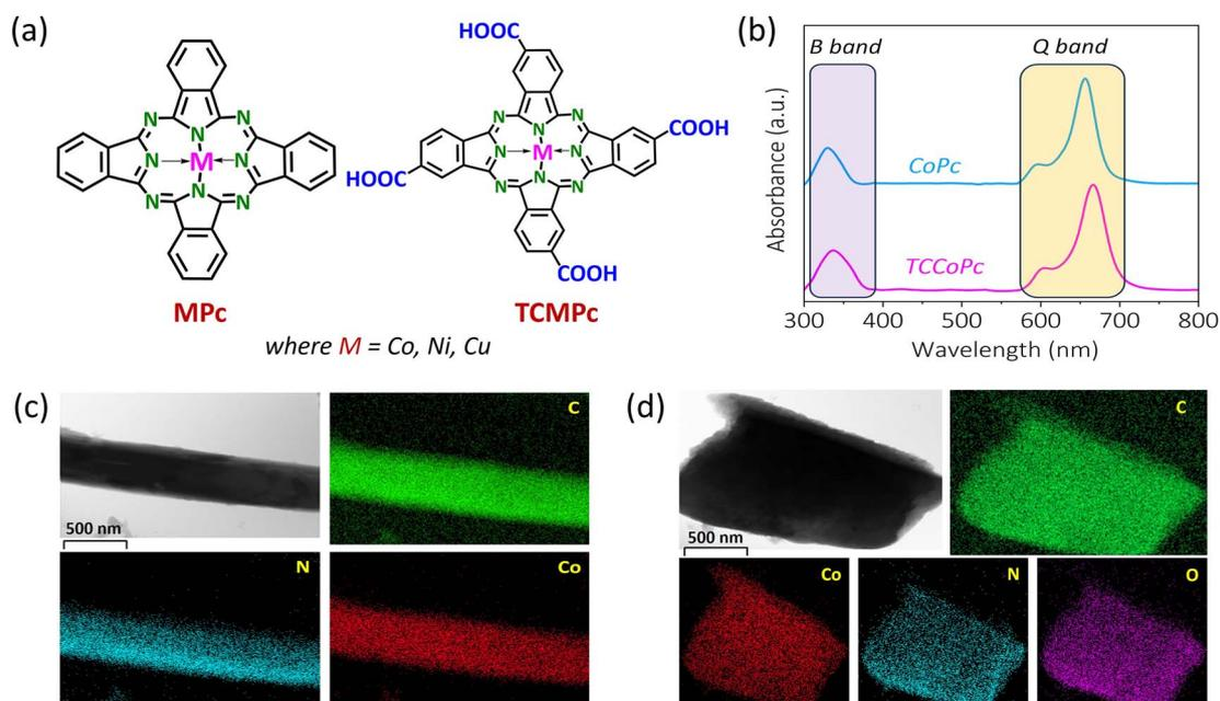
Fig. 1 (a) Molecular structures of unsubstituted metal phthalocyanine (MPc) and tetra-carboxy-substituted metal phthalocyanine (TCMPc), where  $M = \text{Co}, \text{Ni}, \text{Cu}$ . (b) UV-visible spectra of CoPc and TCCoPc molecules. HRTEM images along with elemental mapping of (c) CoPc and (d) TCCoPc molecules.
