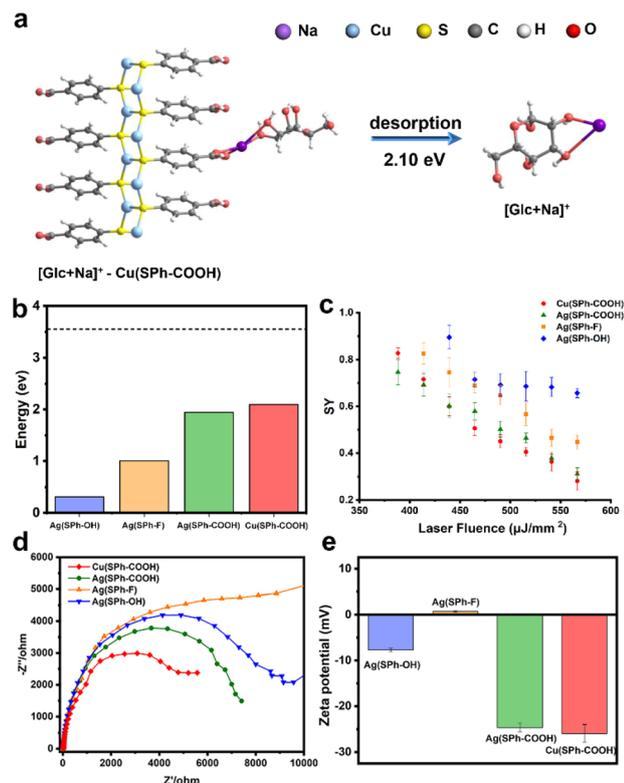
Fig. 3 (a) Desorption of  $[\text{Glc} + \text{Na}]^+$  from  $\text{Cu}(\text{SPh}-\text{COOH})$  surface simulated by DFT, (b) the desorption energies of  $[\text{Glc} + \text{Na}]^+$  from the four OMCs (the dotted line represents the laser energy (3.55 eV) used for LDI-MS), (c) effect of laser fluence on the SY value of 4-MeBP<sup>+</sup> with the four few-layered OMCs as substrates, and (d) EIS and (e) zeta potential of the four few-layered OMCs.
