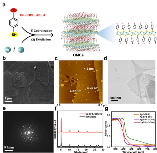
Fig. 1 (a) Scheme of preparation for few-layered OMCs; (b) SEM image, (c) AFM image, (d) TEM image, (e) corresponding SAED pattern, and (f) PXRD pattern of Cu(SPh-COOH) nanosheets; (g) UV-vis spectra of the four few-layered OMCs (the dotted line represented the laser wavelength (355 nm) used for LDI-MS).
