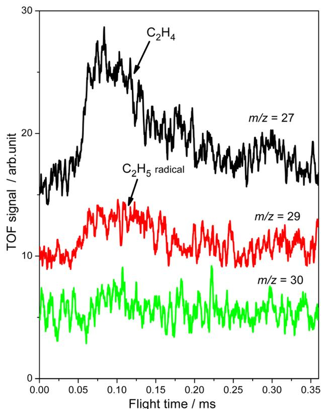
Fig. 3 The TOF signals of  $C_2H_4$  collected at  $m/z = 27$  ( $C_2H_3^+$ ), 29 ( $C_2H_5^+$ ) and 30 ( $C_2H_6^+$ ) as a function of the flight time when irradiating the 0.28 ML  $C_2H_6$  covered oxidized R-TiO<sub>2</sub>(110) surfaces at 343 nm. The photon flux of the 343 nm light is  $2.0 \times 10^{16}$  photons per cm<sup>2</sup> per s.
