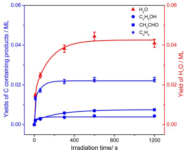
Fig. 5 The yields of H<sub>2</sub>O (red triangles) and carbon containing products (C<sub>2</sub>H<sub>5</sub>OH (blue circles), CH<sub>3</sub>CHO (blue squares), and C<sub>2</sub>H<sub>4</sub> (blue stars)) in photocatalytic ODHE on oxidized R-TiO<sub>2</sub>(110) as a function of irradiation time, derived from Fig. 4. All the plotted lines are only to guide the eye.
