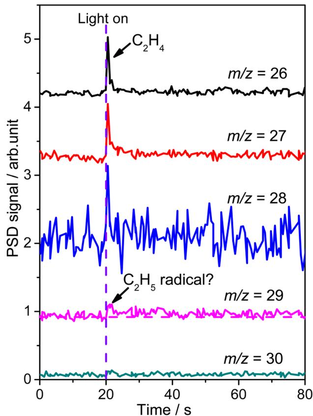
Fig. 2 The PSD spectra acquired at  $m/z = 26$  ( $C_2H_2^+$ ),  $27$  ( $C_2H_3^+$ ),  $28$  ( $C_2H_4^+$ ),  $29$  ( $C_2H_5^+$ ) and  $30$  ( $C_2H_6^+$ ) on the 0.28 ML  $C_2H_6$  covered oxidized R-TiO<sub>2</sub>(110) surfaces. The purple dashed line represents the moment when the light is turned on ( $t = 20$  s). The photon flux of the 355 nm light is  $2.4 \times 10^{16}$  photons per  $cm^2$  per s.
