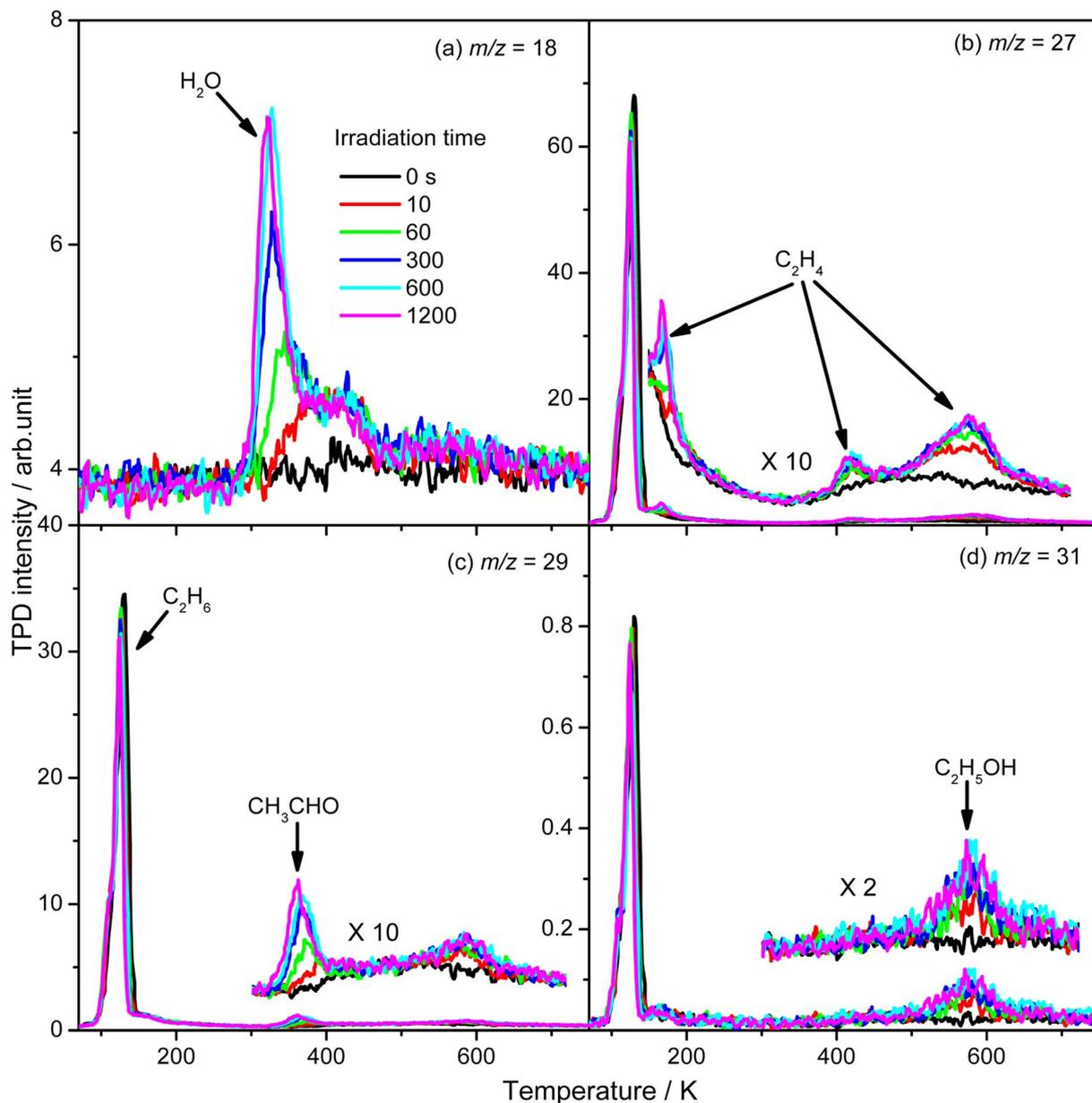
Fig. 4 The TPD spectra acquired at  $m/z = 18$  ( $\text{H}_2\text{O}^+$ ) (a), 27 ( $\text{C}_2\text{H}_3^+$ ) (b), 29 ( $\text{C}_2\text{H}_5^+$ ) (c), and 31 ( $\text{CH}_3\text{O}^+$ ) (d) on the 0.28 ML  $\text{C}_2\text{H}_6$  covered oxidized R- $\text{TiO}_2(110)$  surfaces as a function of irradiation time. The desorption peaks of the carbon containing products are been highlighted in the inserts of (b–d).
