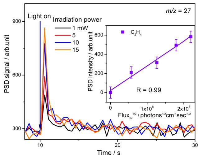
Fig. 6 The PSD signals of C<sub>2</sub>H<sub>4</sub> collected from the 0.28 ML C<sub>2</sub>H<sub>6</sub> covered oxidized R-TiO<sub>2</sub>(110) surfaces as a function of the laser irradiation power. The intensity of the PSD signals (the initial point when the UV light is turned on) of C<sub>2</sub>H<sub>4</sub> has a linear relationship with the square root of the incident light flux ( $F_{hv}^{1/2}$ ), as shown in the inset of this figure.
