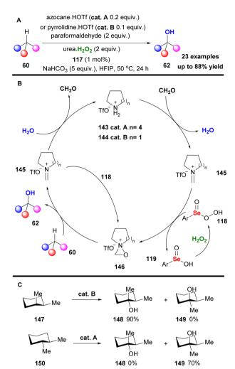
Scheme 34 (A) C-H hydroxylation employing the in situ generated iminium salt 145. (B) Studies on the retention of stereochemistry. (C) Hydroxylation of cyclohexanes.
