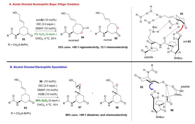
Scheme 23 Catalyst dependent chemoseletive oxidations of bifunctional substrates using (A) ent-83 or (B) 96.
