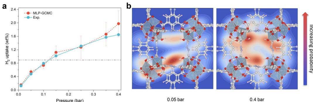
Fig. 4 MLP-GCMC prediction. (a) Simulated  $\text{H}_2$  adsorption isotherms for Al-soc-MOF-1d (red symbols) vs. experimental volumetric measurements (blue symbols) at 77 K, ranging from 0.01 to 0.4 bar. (b) Simulated probability distribution of  $\text{H}_2$  at 0.05 (left) and 0.4 bar (right), respectively.
