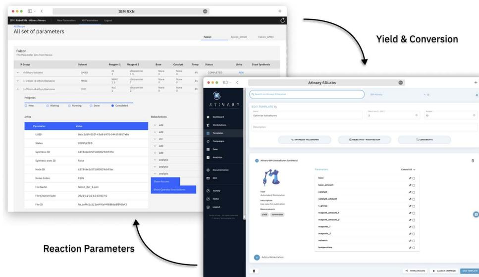
**Fig. 3** The graphical user interface of the Atinary SDLabs and the frontend application. SDLabs allows the user to configure the optimization campaign, while the frontend facilitates the execution of the reaction and reporting of the measured yields and conversions.
