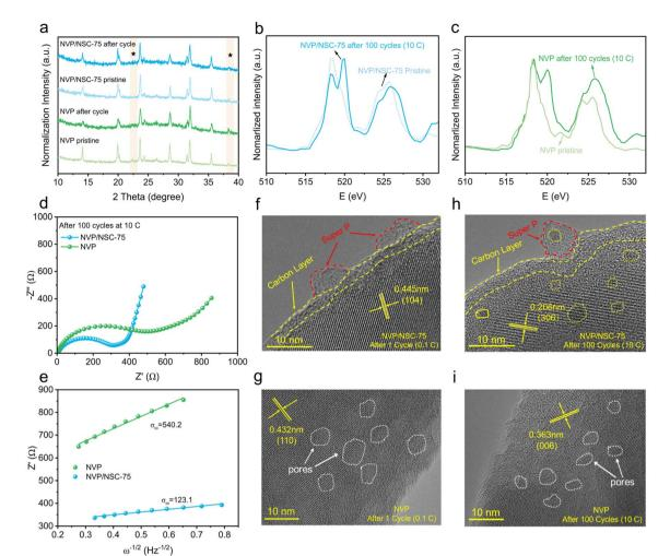
Fig. 8 (a) Ex situ XRD patterns of NVP and NVP/NSC-75 before and after cycling. (b and c) Normalized sXAS spectra of NVP and NVP/NSC-75 after cycling. (d) Nyquist plots of samples after 100 cycles at 10C. (e) The relationship between Z' and  $\omega^{-1/2}$  after 100 cycles at 10C. (f–i) HRTEM images of NVP and NVP/NSC-75 samples after cycling.
