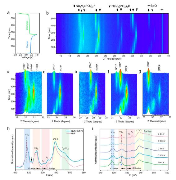
Fig. 7 (a) GCD curves of NVP/NSC-75. (b) *In situ* XRD patterns and (c–g) structural evolution of the NVP/NSC-75 electrode during the extraction/intercalation of Na<sup>+</sup>. (h) Normalized sXAS spectra of the V L-edge and O K-edge for NVP and NVP/NSC-75. (i) Normalized sXAS spectra of NVP/NSC-75 at different charging/discharging states.
