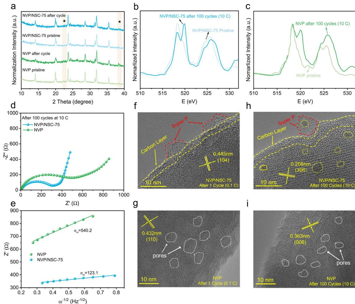
Fig. 8 (a) *Ex situ* XRD patterns of NVP and NVP/NSC-75 before and after cycling. (b and c) Normalized sXAS spectra of NVP and NVP/NSC-75 after cycling. (d) Nyquist plots of samples after 100 cycles at 10C. (e) The relationship between  $Z'$  and  $\omega^{-1/2}$  after 100 cycles at 10C. (f–i) HRTEM images of NVP and NVP/NSC-75 samples after cycling.
