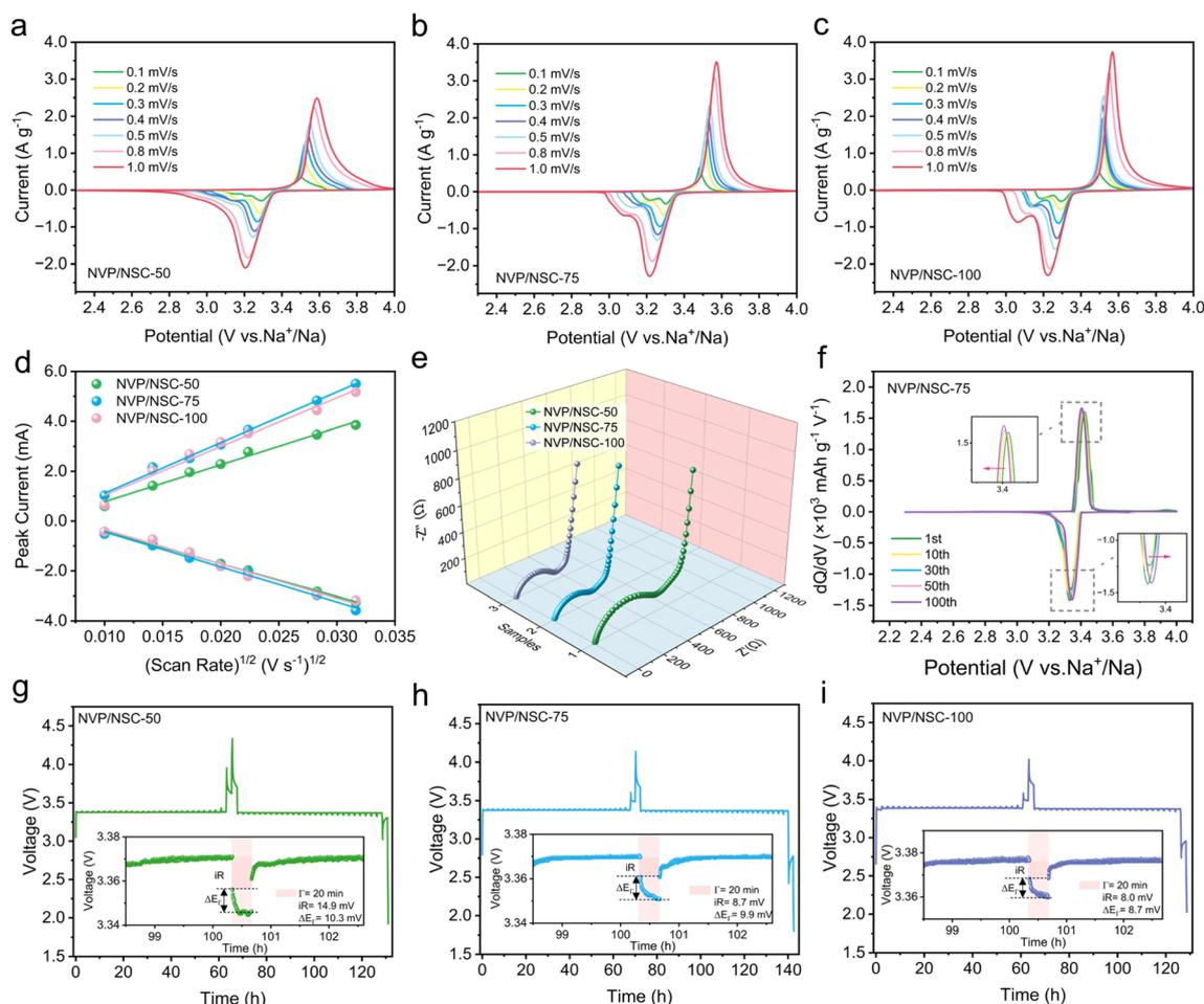
Fig. 6 Kinetic properties of NVP/NSC-50, NVP/NSC-75 and NVP/NSC-100. CV curves at different scanning rates of (a) NVP/NSC-50, (b) NVP/NSC-75, and (c) NVP/NSC-100. (d) Linear fits for the anodic and cathodic peak currents versus scan rates of NVP/NSC samples. (e) Nyquist plots of NVP/NSC samples. (f) The  $dQ/dV$  curves of NVP/NSC-75 for the selected cycles at 1C. (g–i) Transient voltage–time profile obtained from a GITT test for NVP/NSC samples.
