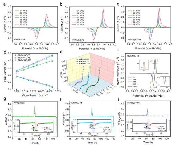
Fig. 6 Kinetic properties of NVP/NSC-50, NVP/NSC-75 and NVP/NSC-100. CV curves at different scanning rates of (a) NVP/NSC-50, (b) NVP/ NSC-75, and (c) NVP/NSC-100. (d) Linear fits for the anodic and cathodic peak currents versus scan rates of NVP/NSC samples. (e) Nyquist plots of NVP/NSC samples. (f) The dQ/dV curves of NVP/NSC-75 for the selected cycles at 1C. (g-i) Transient voltage-time profile obtained from a GITT test for NVP/NSC samples.
