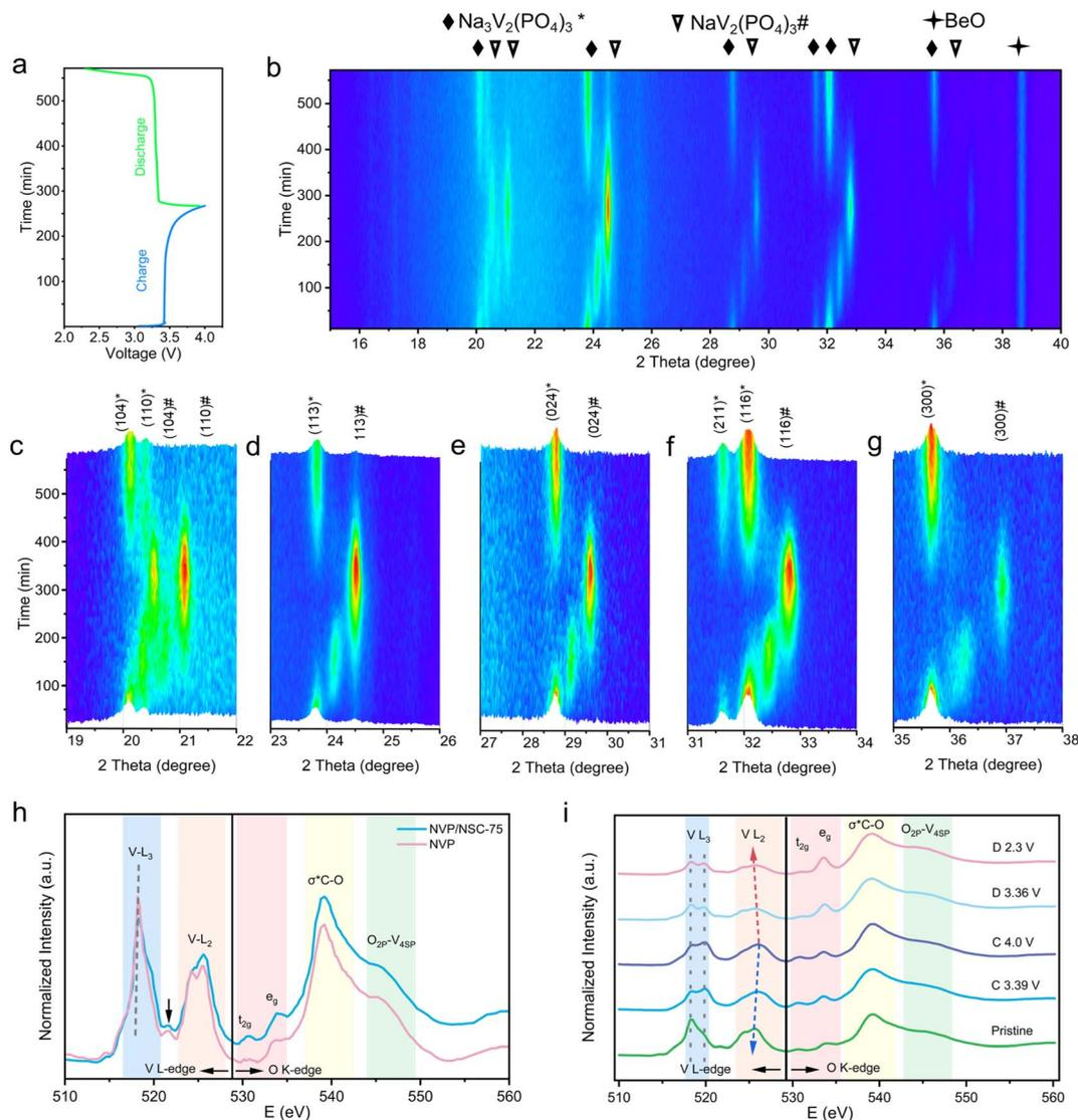
Fig. 7 (a) GCD curves of NVP/NSC-75. (b) *In situ* XRD patterns and (c–g) structural evolution of the NVP/NSC-75 electrode during the extraction/intercalation of  $\text{Na}^+$ . (h) Normalized sXAS spectra of the V L-edge and O K-edge for NVP and NVP/NSC-75. (i) Normalized sXAS spectra of NVP/NSC-75 at different charging/discharging states.
