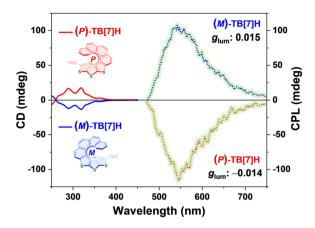
Fig. 5 Chiroptical properties. CD (dashed curves) and CPL (dot curves) spectra of enantiomers (M)-TB[7]H and (M)-TB[7]H. Both samples were characterized in the solution of 2-MeTHF with a concentration of 5  $\times$  10<sup>-5</sup> M. The CD spectra were recorded at room temperature, while the CPL spectra were detected at 77 K.
