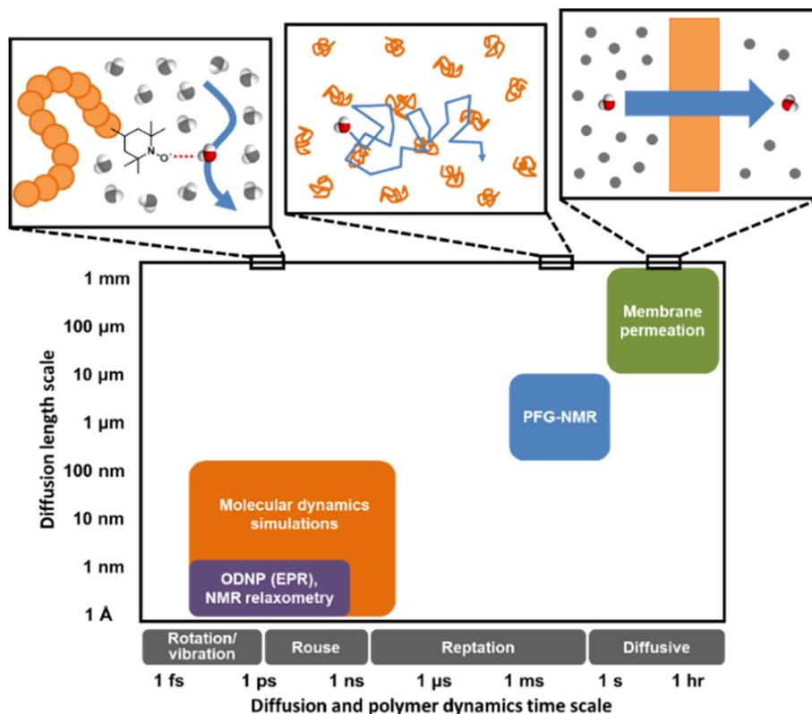
Fig. 1 Distinct experimental and computational techniques probe small molecule diffusion processes occurring over vastly different length and time scales.<sup>43</sup> Techniques such as MD simulations and ODNP can uncover molecular-scale dynamic behavior of small molecules in polymers or polymer solutions while tools like PFG-NMR and membrane permeation experiments reveal macroscopic transport phenomena.
