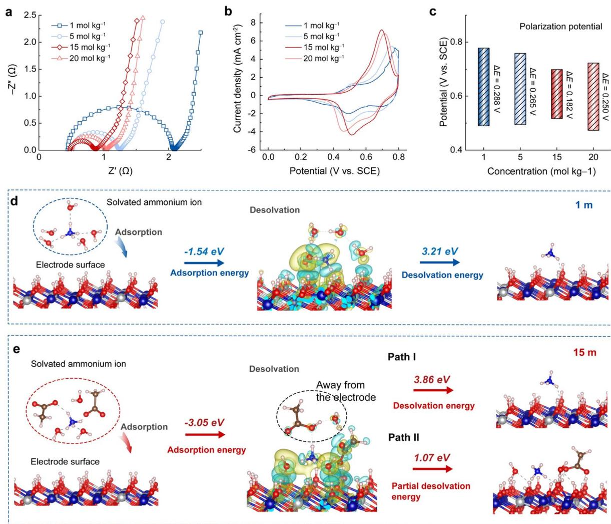
Fig. 3 (a) Nyquist plots of the A-CoNi DH electrode in different concentrated  $\text{CH}_3\text{COONH}_4$  electrolytes. (b) CV curves of the A-CoNi DH electrodes in different electrolytes at the scan rate of  $0.5 \text{ mV s}^{-1}$ . (c) The redox polarization potentials of A-CoNi DH's CV curves (b) in different electrolytes. The simulated electrolyte–electrode interface processes upon discharging in (d) 1 m, and (e) 15 m  $\text{CH}_3\text{COONH}_4$  electrolytes, respectively.
