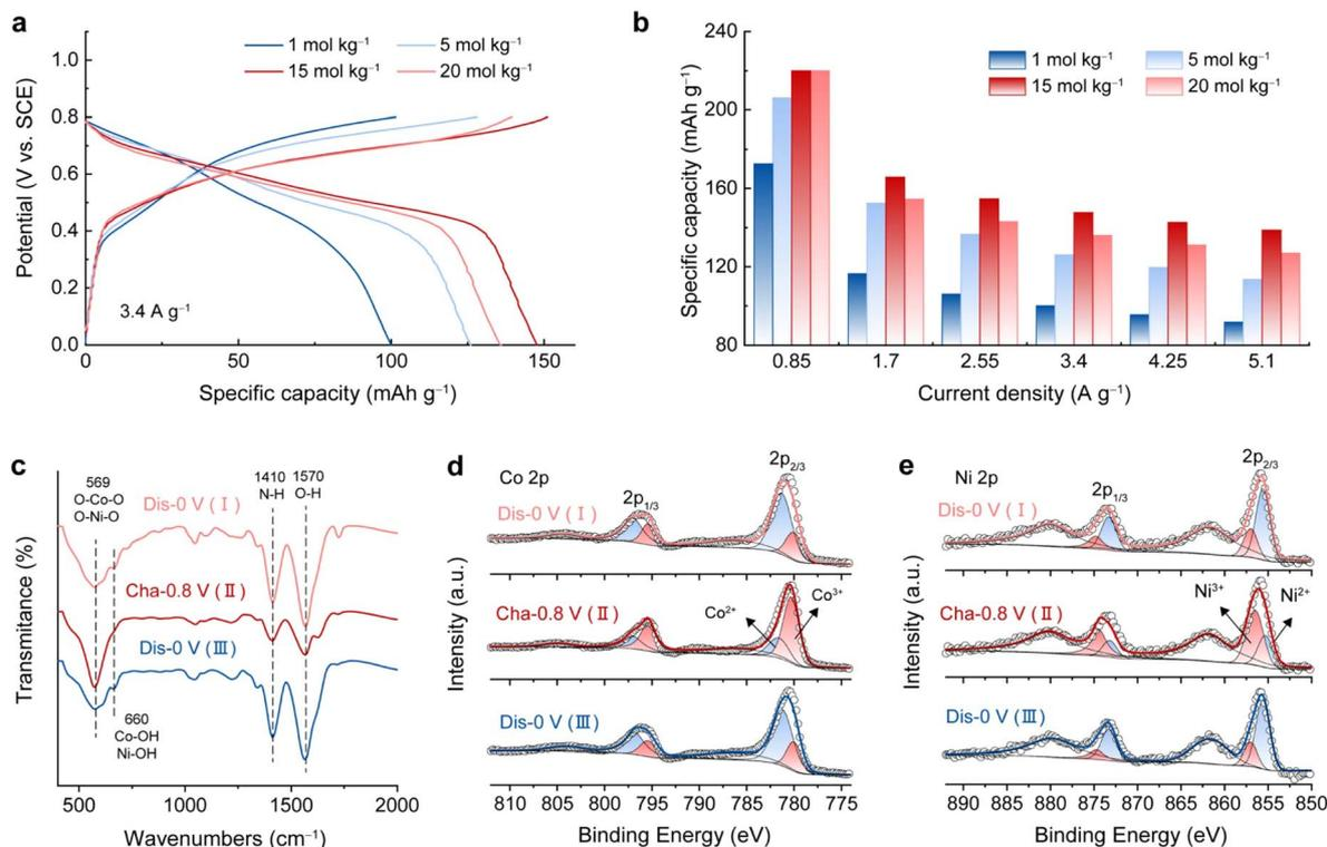
Fig. 1 (a) Galvanostatic charge/discharge curves of the A-CoNi DH electrode in different concentrations of ammonium acetate electrolyte at the current density of  $3.4 \text{ A g}^{-1}$ . (b) Rate performance of the A-CoNi DH electrode in different states of charge. (c) FTIR, (d) XPS Co 2p, and (e) XPS Ni 2p spectra of the A-CoNi DH electrode at different states of charge.
