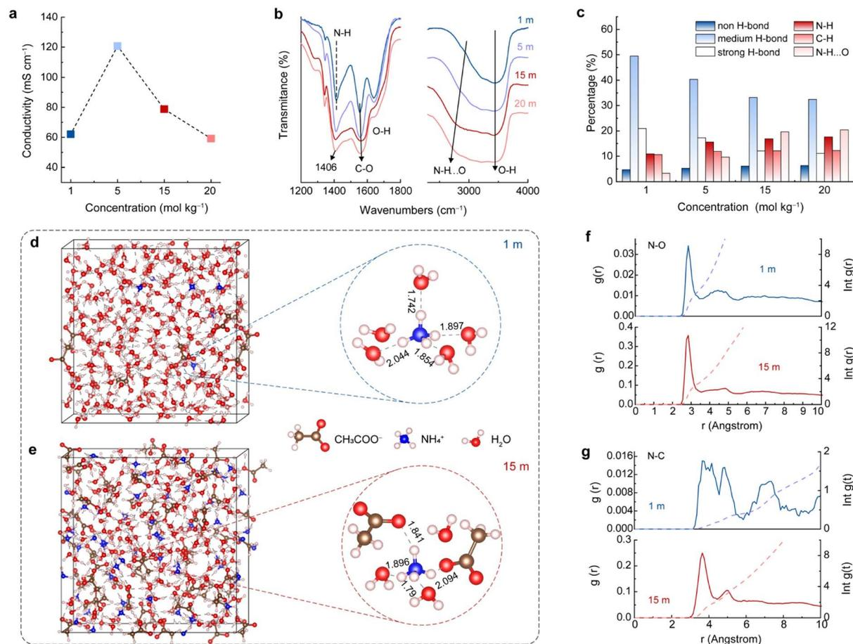
Fig. 2 (a) Electrical conductivity and (b) FTIR spectra of  $\text{CH}_3\text{COONH}_4$  electrolytes with different concentrations. (c) The corresponding percentage of the chemical bonds summarized in Fig. S9.† (d) and (e) MD simulation. (f) and (g) RDF plots of N–O and N–C, and the corresponding average coordination number of 1 and 15 m  $\text{CH}_3\text{COONH}_4$  electrolytes.
