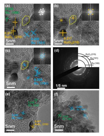
Fig. 2 (a-c) HRTEM images of Ru/CC (-0.8 to 1.1 V) and the corresponding FFT patterns. (d) SAED pattern of Ru/CC (-0.8 to 1.1 V). HRTEM images of (e) Ru/CC (0-1.1 V) and (f) Ru/CC (-0.8 to 0 V).
