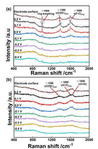
Fig. 7 In situ Raman spectra collected on the Ru/CC (-0.8 to 1.1 V) surface for (a) benzoate and (b) cyclohexene carboxylate in 0.1 M KOH at different applied potentials.
