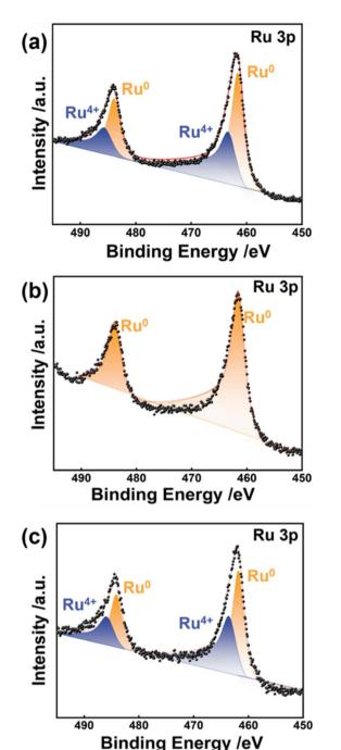
Fig. 3 Ru 3p XPS spectra of (a) Ru/CC (-0.8 to 1.1 V), (b) Ru/CC (-0.8 to 0 V), and (c) Ru/CC (0-1.1 V).
