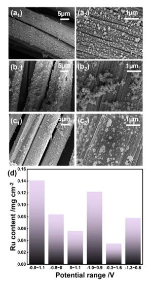
Fig. 1 SEM images of (a) Ru/CC (-0.8 to 1.1 V), (b) Ru/CC (-0.8 to 0 V), and (c) Ru/CC (0-1.1 V). (d) The mass loading of Ru for Ru/CC (-0.8 to 1.1 V), Ru/CC (-0.8 to 0 V), Ru/CC (0-1.1 V), Ru/CC (-1.0 to 0.9 V), Ru/ CC (-0.3 to 1.6 V) and Ru/CC (-1.3 to 0.6 V).
