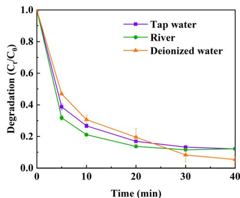
Fig. 10 OTC degradation catalyzed by the HCN-500/PDS system in river water and tap water. Conditions: 20  $\text{mg L}^{-1}$  of OTC, 0.5  $\text{g L}^{-1}$  of HCN-500, 0.1  $\text{g L}^{-1}$  of PDS at 30 °C.
