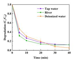
Fig. 10 OTC degradation catalyzed by the HCN-500/PDS system in river water and tap water. Conditions: 20 mg L $^{-1}$  of OTC, 0.5 g L $^{-1}$  of HCN-500, 0.1 g L $^{-1}$  of PDS at 30 °C.
