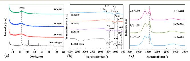
Fig. 1 (a) XRD, (b) FT-IR and (c) Raman spectra of HCNs.
