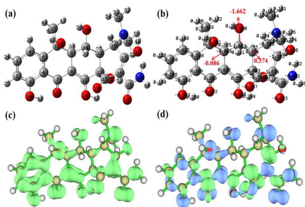
Fig. 7 Optimal structure of OTC with (a) atomic number, (b) optimal structure with Mulliken charge, and (c) isosurfaces of the Fukui function  $f^-$  and (d) dual descriptor. Green: positive; blue: negative, iso-surface value = 0.001 a.u. of OTC.
