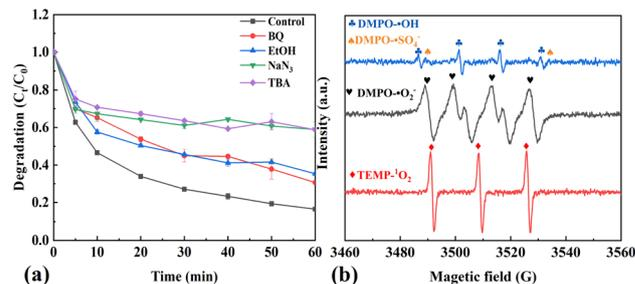
Fig. 6 (a) Effect of benzoquinone (BQ, 0.4 mM), NaN<sub>3</sub> (0.4 mM), EtOH (1.6 M) and tertiary butyl alcohol (TBA, 0.4 mM) on OTC degradation over HCN-500/PDS; (b) EPR spectra of HCN-500/PDS system. Conditions: 20 mg L<sup>-1</sup> of OTC, 0.25 g L<sup>-1</sup> of HCN-500, 0.1 g L<sup>-1</sup> of PDS at 30 °C.
