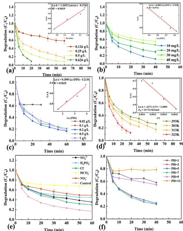
Fig. 5 Influences of (a) HCN-500 amounts, (b) initial OTC concentration, (c) PDS concentration, (d) degradation temperature, (e) anion, and (f) pH on OTC degradation. Reaction conditions: 20 mg L<sup>-1</sup> of OTC, 0.25 g L<sup>-1</sup> of HCN-500, 0.1 g L<sup>-1</sup> of PDS and 20 mM anion at 30 °C.
