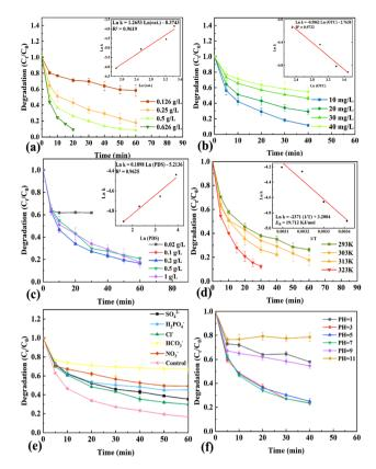
Fig. 5 Influences of (a) HCN-500 amounts, (b) initial OTC concentration, (c) PDS concentration, (d) degradation temperature, (e) anion, and (f) pH on OTC degradation. Reaction conditions: 20 mg  $L^{-1}$  of OTC, 0.25 g  $L^{-1}$  of HCN-500, 0.1 g  $L^{-1}$  of PDS and 20 mM anion at 30 ° C.
