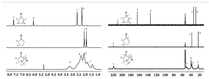
Fig. 1 <sup>1</sup>H-NMR (left) and <sup>13</sup>C(<sup>1</sup>H) NMR spectra (right) in parts per million (ppm) of the monomer (top), the repeating unit motif (middle), and the polymer (bottom) in deuterated dichloromethane.
