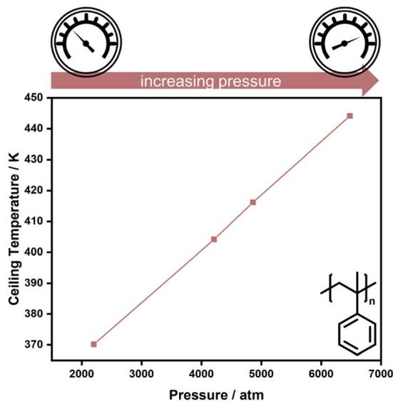
Fig. 3 High pressure increases the ceiling temperature in the polymerization of  $\alpha$ -methyl styrene. Adapted from ref. 74 with permission from the Royal Society of Chemistry, copyright 1960.
