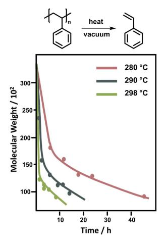
Fig. 9 Change of molecular weight of PS during the depolymerization at different temperatures. Adapted from ref. 86 with permission from the Royal Society of Chemistry, copyright 1957.
