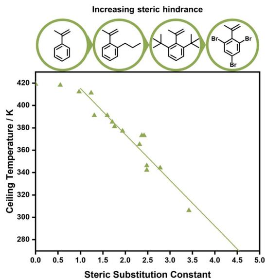
Fig. 4 The effect of phenyl methacrylate's substituents on the ceiling temperature, the larger the substituent the lower the ceiling temperature of the polymerization. Graph reprinted from ref. 90 *Eur. Polym. J.*, 25, 2, B. Yamada, T. Tanaka, T. Otsu, Correlations of ceiling temperature and reactivity with bulkiness of *ortho*-substituent in radical polymerization of phenyl methacrylate, 117–120, Copyright 1989, with permission from Elsevier.
