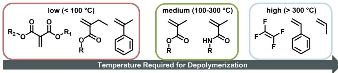
Fig. 6 Temperature required for depolymerization of vinyl monomers, the further to the right the monomer is, the higher the required temperature to effectively depolymerize its corresponding polymer.
