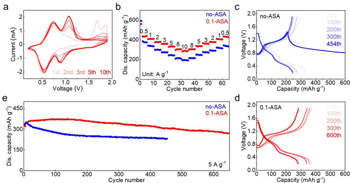
Fig. 5 Electrochemical performance of the  $V_6O_{13} \cdot H_2O$  cathode in the  $ZnSO_4$  electrolyte without and with a 0.1 m ASA additive. (a) CV curves in 0.1-ASA. (b) Rate performance in the two electrolytes. Charge–discharge curves at different cycles in (c)  $ZnSO_4$  and (d) 0.1-ASA, and (e) the capacity evolution at  $5 A g^{-1}$ .
