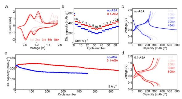
Fig. 5 Electrochemical performance of the  $V_6O_{13} \cdot H_2O$  cathode in the ZnSO<sub>4</sub> electrolyte without and with a 0.1 m ASA additive. (a) CV curves in 0.1-ASA. (b) Rate performance in the two electrolytes. Charge-discharge curves at different cycles in (c) ZnSO<sub>4</sub> and (d) 0.1-ASA, and (e) the capacity evolution at 5 A g<sup>-1</sup>
