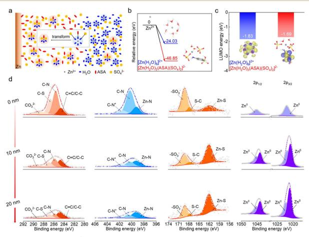
Fig. 3 (a) Schematic illustrations of Zn<sup>2+</sup> solvation structures in the bulk electrolyte and at the interface. (b) The relative energies for the formation of  $[Zn(H_2O)_6]^{2+}$  and  $[Zn(H_2O)_3(ASA)(SO_4)_2]^{2-}$ . (c) The LUMO energy levels and orbitals of  $[Zn(H_2O)_6]^{2+}$  and  $[Zn(H_2O)_3(ASA)(SO_4)_2]^{2-}$ . (d) The C 1s, N 1s, S 2p and Zn 2p XPS with different sputtering depths of the electro-deposited Zn from the 0.1-ASA electrolyte.
