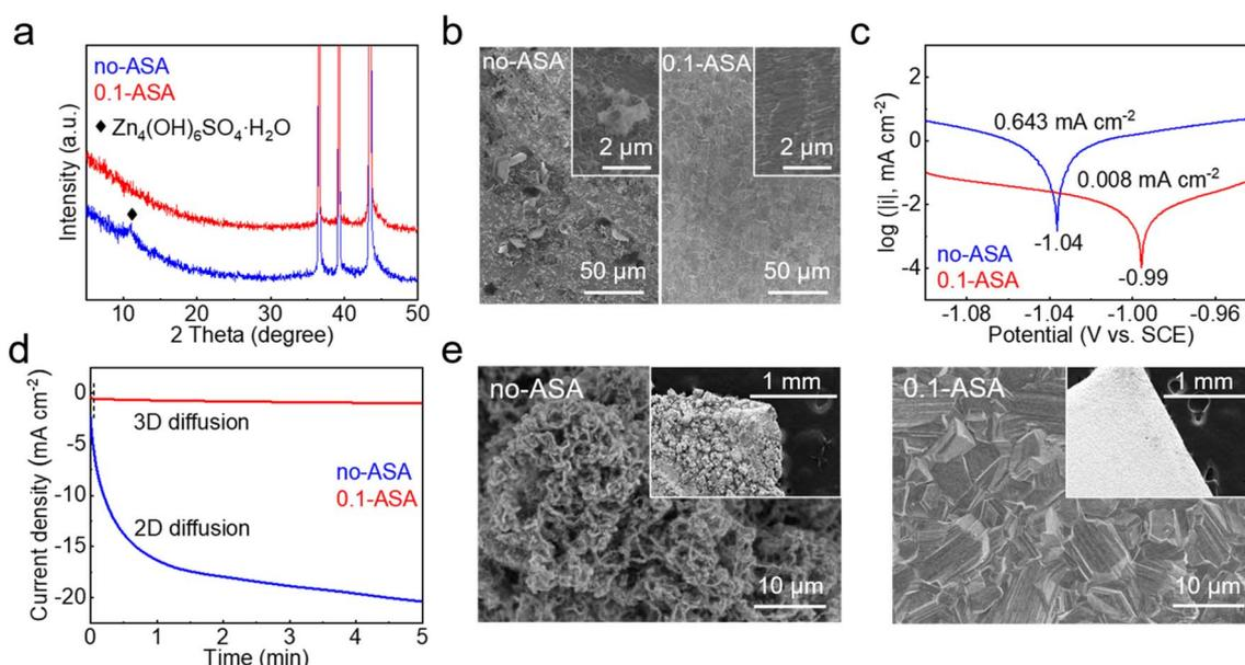
Fig. 4 (a) XRD patterns and (b) SEM images of Zn after soaking in the two solutions for 24 h. (c) Tafel plots and (d) CA curves at  $-150 \text{ mV vs. Zn}$  constant potential in the two electrolytes. (e) SEM images of the electro-deposited Zn (at  $10 \text{ mA cm}^{-2}$  for 1.5 h) in the two electrolytes.
