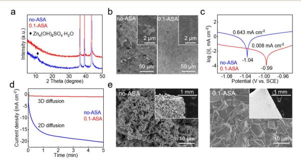
Fig. 4 (a) XRD patterns and (b) SEM images of Zn after soaking in the two solutions for 24 h. (c) Tafel plots and (d) CA curves at -150 mV vs. Zn constant potential in the two electrolytes. (e) SEM images of the electro-deposited Zn (at 10 mA cm<sup>-2</sup> for 1.5 h) in the two electrolytes.
