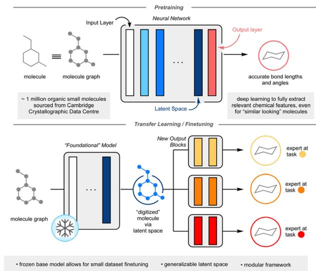
**Fig. 1** Graphical overview of the framework. Top panel illustrates the pretraining process and the structure of deep learning neural networks. The bottom panel shows how the top large model (foundational model) can be used for new chemistry-relevant predictions via the foundational model's latent space.
