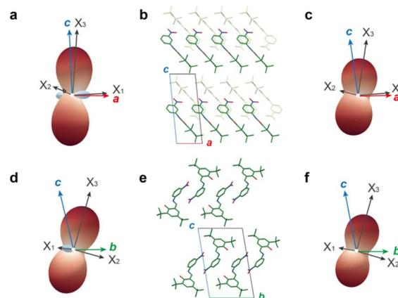
Fig. 4 (a, c, d and f) Expansivity indicatrices obtained from PASCAL<sup>22</sup> in the temperature range (a and d) from  $-1.6$  to  $23.6$  °C and (c and f) from  $32.0$  to  $57.2$  °C viewed from the (a and c) (010) and (d and f) (100) faces, respectively. Red and blue represent positive and negative thermal expansion, respectively. (b and e) Molecular packing viewed from the (b) (010) and (e) (100) faces, respectively.
