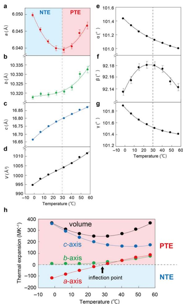
Fig. 3 Temperature dependence of unit cell parameters of the enol-1 crystal: (a)  $a$ -axis, (b)  $b$ -axis, (c)  $c$ -axis, (d) volume, (e)  $\alpha$ -angle, (f)  $\beta$ -angle, and (g)  $\gamma$ -angle. In (c–e and g) the error bars are hidden behind plots. (h) Temperature dependence of the coefficients of thermal expansion (CTEs) of the three axes and the cell volume.
