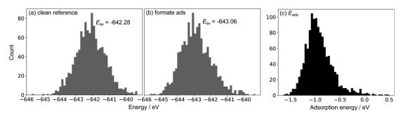
Fig. 2 Sample energy distributions for (a) clean Ga-In at 450 K (standard deviation: 0.76 eV). Note that a reference energy of  $E_{CO_2} + \frac{1}{2}E_{H_2}$  has been added to allow direct comparison to the formate-adsorbed surface. (b) The energy distribution for Ga-In with formate adsorbed to the surface at 450 K (standard deviation: 0.86 eV). (c) The adsorption energy of formate calculated by subtracting clean energies from adsorbed energies in a matching point-by-point fashion.
