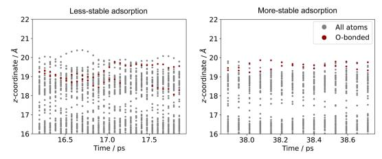
Fig. 5 The z-coordinates of metal atoms in the surface layers of Ga-In with formate adsorbed. The Ga atoms which are bonded to O are shown in red. The O-bonded Ga on the surface are seen to be more elevated in the low energy region than the high.
