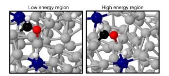
Fig. 8 A comparison of structures from the stable (left) and unstable (right) adsorption regions for liquid metal sampling of the \*CHO + \*3H state. The most pronounced difference is the elevation of Ga atoms underneath the adsorbates. Key: Ga-silver, Pt-blue, O-red, C-black, Hwhite
