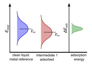
Fig. 1 An example schematic showing sampled energies of an attemperature clean liquid metal (blue), and a liquid metal with the adsorbate present (red). In this example, the adsorbed state is, on average, more stable than the clean liquid metal. The calculated adsorption energies also have a range, denoted by the green curve. Note that, for clarity, the energy of the adsorbate in a box (which is a constant) has been added to the blue curve so that each system has the same atoms accounted for.
