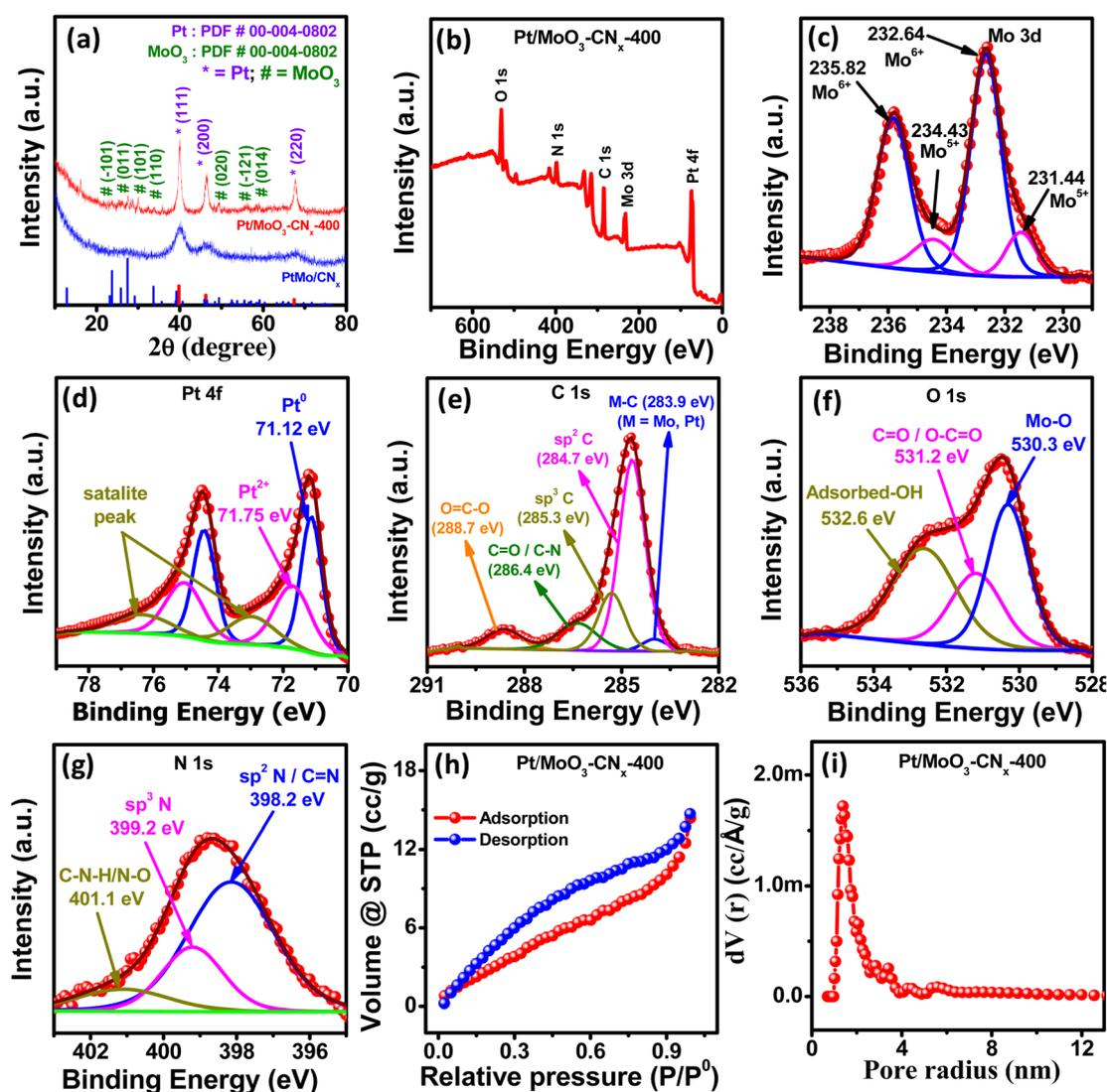
Fig. 2 (a) p-XRD spectra of Pt/MoO<sub>3</sub>-CN<sub>x</sub>-400 and PtMo/CN<sub>x</sub>. (b) XPS survey scan spectrum of Pt/MoO<sub>3</sub>-CN<sub>x</sub>-400. (c-g) High-resolution XPS spectra of Mo 3d, Pt 4f, C 1s, O 1s, and N 1s for Pt/MoO<sub>3</sub>-CN<sub>x</sub>-400, respectively. (h and i) N<sub>2</sub> physisorption isotherm and pore size distribution plots for Pt/MoO<sub>3</sub>-CN<sub>x</sub>-400, respectively.
