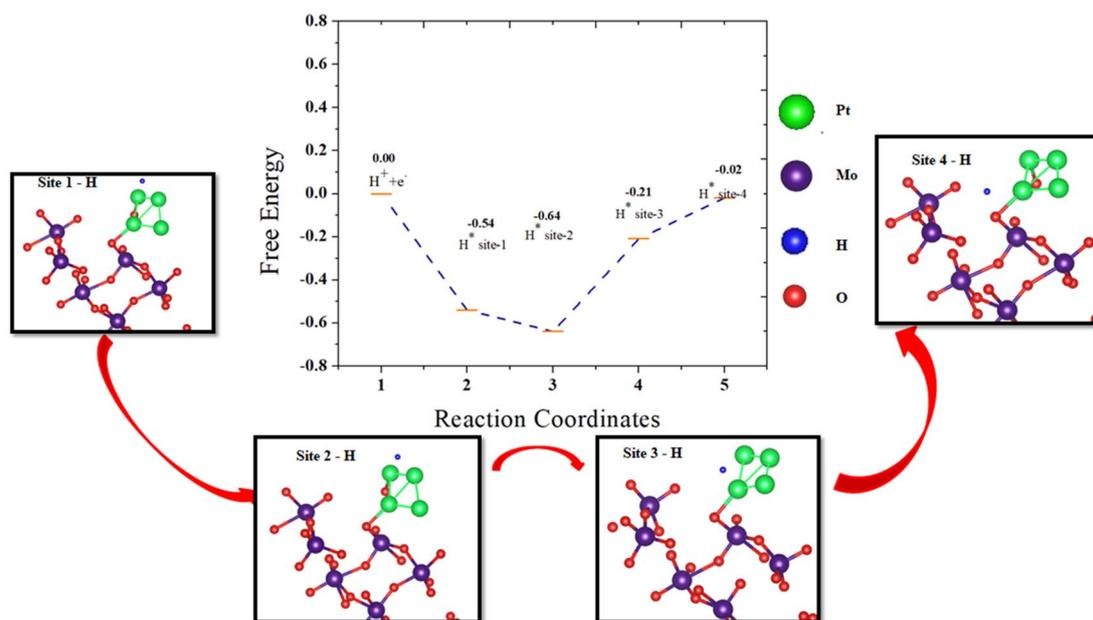
Fig. 8 Schematic presentation of a free energy diagram for the HER on the surface of Pt@MoO<sub>3</sub> (011). Optimized H\* adsorption structures from site 1 to site 4 at different locations on Pt@MoO<sub>3</sub> (011) are shown in the black boxes according to the red arrows.
