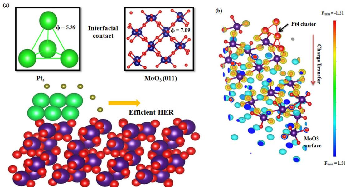
Fig. 7 (a) Schematic illustration of the hydrogen spillover mechanism over a Pt<sub>4</sub>@MoO<sub>3</sub> (011) surface. (b) Charge density difference plot across the Pt<sub>4</sub>@MoO<sub>3</sub> (011) surface.
