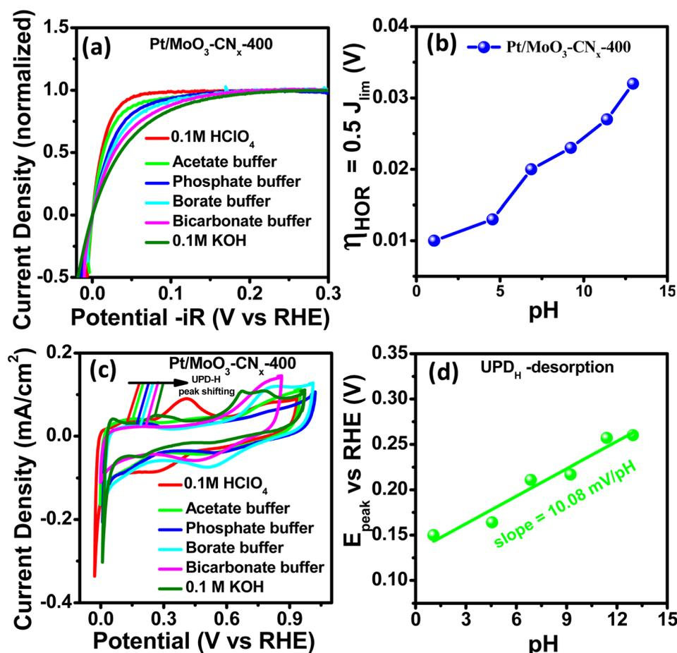
Fig. 5 (a) Normalized HOR plots for Pt/MoO<sub>3</sub>-CN<sub>x</sub>-400 in different pH solutions. (b) Overpotential at  $0.5 \times J_{\text{lim}}$  vs. pH plot of the catalyst. (c) CV curves for Pt/MoO<sub>3</sub>-CN<sub>x</sub>-400 in different pH solutions. (d)  $E_{\text{peak}}$  of UPD-H vs. pH plot of Pt/MoO<sub>3</sub>-CN<sub>x</sub>-400.
