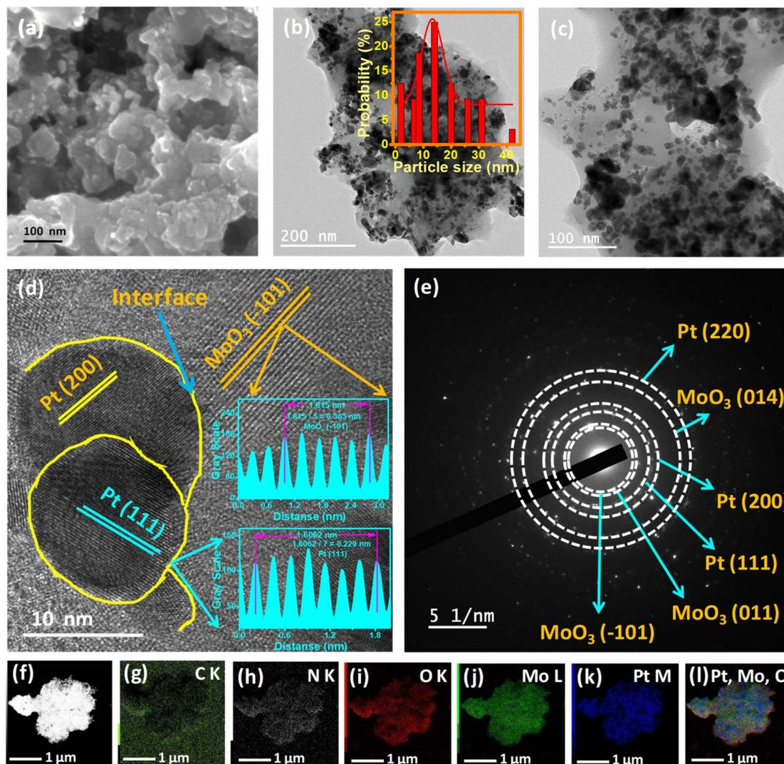
Fig. 1 (a) FE-SEM, (b and c) TEM, (d) HRTEM, and (e) SAED images of Pt/MoO<sub>3</sub>-CN<sub>x</sub>-400. (f–k) STEM and elemental mapping images of Pt/MoO<sub>3</sub>-CN<sub>x</sub>-400. (l) Elemental mapping overlay of Pt, Mo, and O.
