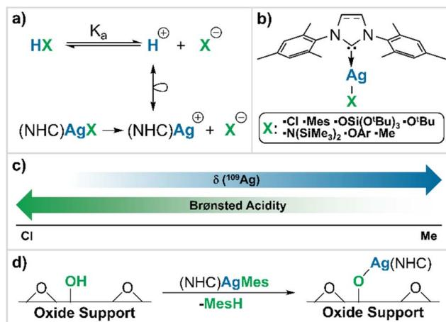
**Scheme 1** General approach to the determination of a correlation between  $\delta^{109}\text{Ag}$  and Brønsted acidity of the conjugate acid of the studied X-type ligands. (a) Isolobal analogy between Brønsted acid HX and the corresponding (NHC)AgX complex; (b) series of (NHC)AgX complexes explored in this work; (c) general trends between Brønsted acidity and  $\delta^{109}\text{Ag}$ ; (d) grafting reaction of the molecular probe onto a generic oxide support.
