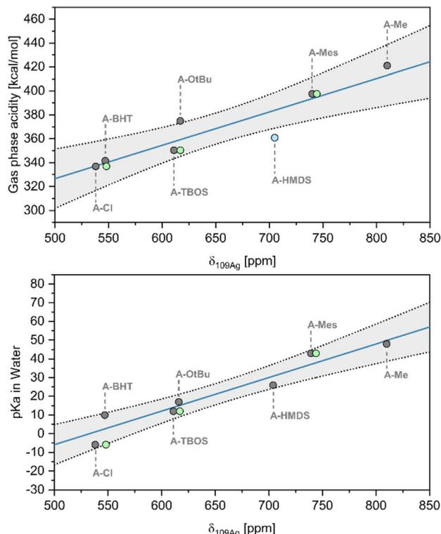
Fig. 2 Linear correlations between  $\delta_{^{109}\text{Ag}}$  and calculated gas phase acidity (DPE) ([top] ( $R^2 = 0.812$ )) and literature  $\text{pK}_a$  values in  $\text{H}_2\text{O}$  ([bottom] ( $R^2 = 0.906$ )). Grey circles show the saturated complexes (A), and green circles represent unsaturated NHC complexes (B).
