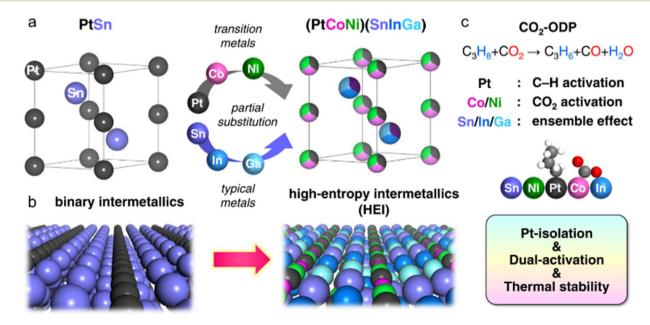
Fig. 5 (a) Catalyst design concept based on the HEI. Pt and Sn sites in intermetallic PtSn (hexagonal NiAs-type structure, space group:  $P6_3/mmc$ ) are partially substituted by Co/Ni and In/Ga, respectively, to form a PtSn-type HEI (PtCoNi) (SnInGa). (b) Atomic arrangement of the most stable (110) surfaces of PtSn (left) and HEI (PtCoNi)(SnInGa) (right). (c) The role of each metal and the effect of multimetallization on the catalysis of CO<sub>2</sub>-ODP.
