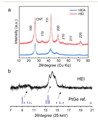
Fig. 6 (a) XRD patterns of the PtRhFeNiCu HEA and HEI catalysts.  $^{23}$  (b) Synchrotron XRD pattern of the (PtCoCu)(GeGaSn)/Ca-SiO $_2$  catalyst.
