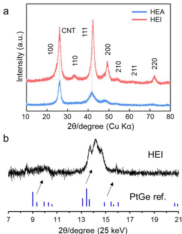
Fig. 6 (a) XRD patterns of the PtRhFeNiCu HEA and HEI catalysts.<sup>23</sup> (b) Synchrotron XRD pattern of the (PtCoCu)(GeGaSn)/Ca-SiO<sub>2</sub> catalyst.
