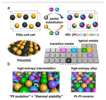
Fig. 3 Catalyst design concept for thermally stable isolated Pt sites using the HEI. (a) Pt and Ge sites in the intermetallic PtGe are partially substituted by Co/Cu and Ge/Sn, respectively, resulting in the formation of the PtGe-type (PtCoCu)(GeGaSn). (b) Illustrations of the (020) surface of the (PtCoCu)(GeGaSn) HEI (left) and the (111) surface of the Pt-based senary HEA (right).
