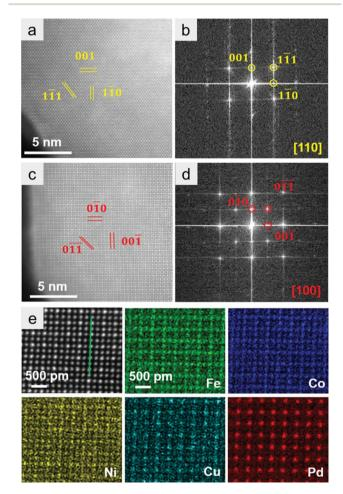
Fig. 7 (a and b) Atom-resolved HAADF-STEM image and the corresponding FFT pattern along the [100] zone axis. (c and d) Atom-resolved HAADF-STEM image and the corresponding FFT pattern along the [110] zone axis. (e) Atom-resolved HAADF-STEM image and corresponding EDS maps. Reproduced with permission from ref. 21. Copyright 2022 Wiley-VCH.
