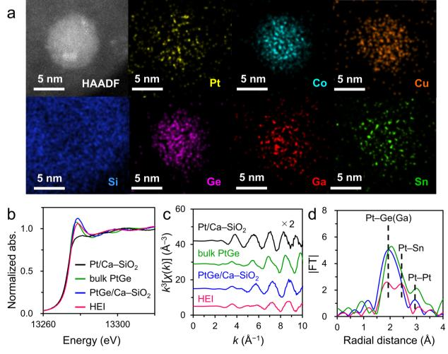
Fig. 8 (a) HAADF-STEM image and the corresponding elemental maps for a single nanoparticle in the (PtCoCu)(GeGaSn)/Ca-SiO<sub>2</sub> catalyst. Pt  $L_{\rm II}$ -edge (b) XANES, (c)  $k^3$ -weighted EXAFS oscillations, and (d) Fourier-transformed EXAFS of Pt/Ca-SiO<sub>2</sub>, bulk PtGe, PtGe/Ca-SiO<sub>2</sub>, and HEI(0.25).
