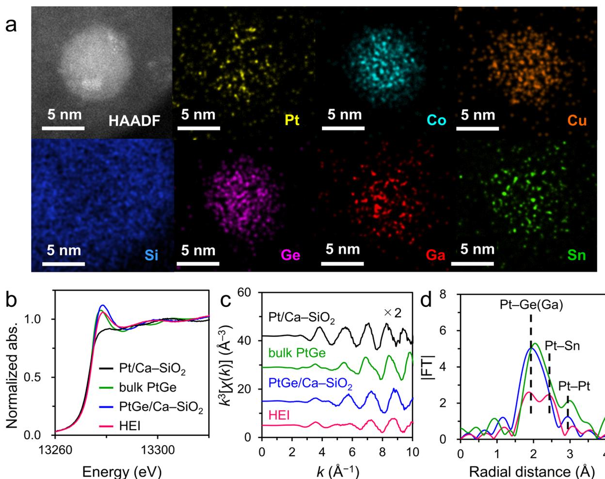
Fig. 8 (a) HAADF-STEM image and the corresponding elemental maps for a single nanoparticle in the  $(\text{PtCoCu})(\text{GeGaSn})/\text{Ca-SiO}_2$  catalyst. Pt  $L_{II}$ -edge (b) XANES, (c)  $k^3$ -weighted EXAFS oscillations, and (d) Fourier-transformed EXAFS of Pt/Ca-SiO<sub>2</sub>, bulk PtGe, PtGe/Ca-SiO<sub>2</sub>, and HEI(0.25).
