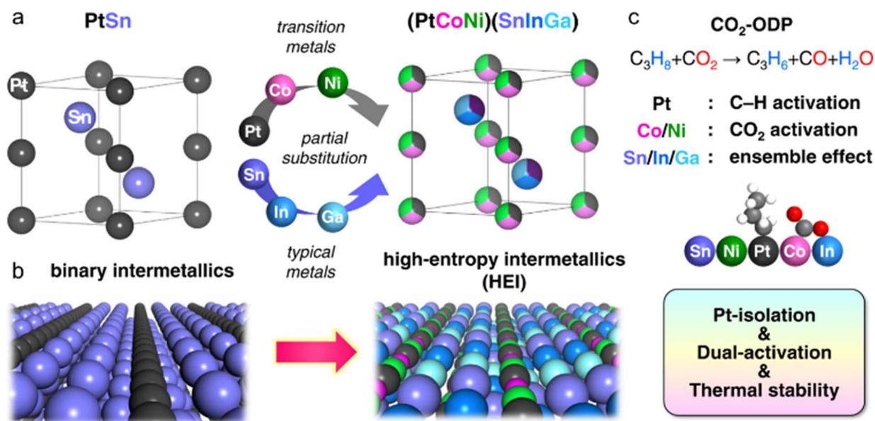
Fig. 5 (a) Catalyst design concept based on the HEI. Pt and Sn sites in intermetallic PtSn (hexagonal NiAs-type structure, space group:  $P6_3/mmc$ ) are partially substituted by Co/Ni and In/Ga, respectively, to form a PtSn-type HEI (PtCoNi)(SnInGa). (b) Atomic arrangement of the most stable (110) surfaces of PtSn (left) and HEI (PtCoNi)(SnInGa) (right). (c) The role of each metal and the effect of multimetalization on the catalysis of CO<sub>2</sub>-ODP.
