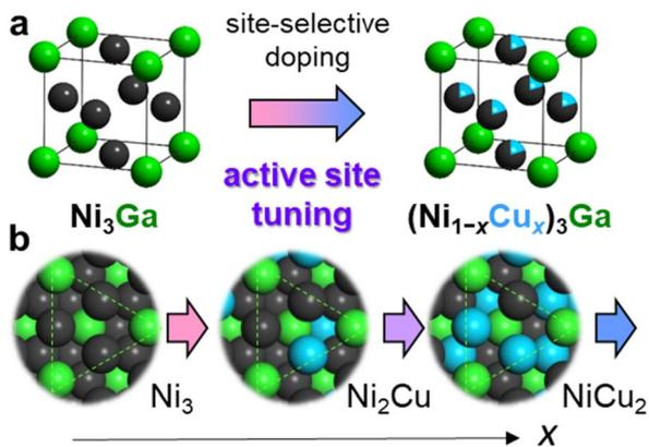
Fig. 1 Active site tuning based on pseudo-binary alloy. (a) Site-selective doping of Cu to the Ni sites of intermetallic  $\text{Ni}_3\text{Ga}$  to form a  $(\text{Ni}_{1-x}\text{Cu}_x)_3\text{Ga}$  pseudo-binary alloy. (b) Atomic arrangement of the  $\text{Ni}_3\text{Ga}$  (111) surface and the changes in the  $\text{Ni}_3$  hollow sites upon Cu substitution.
