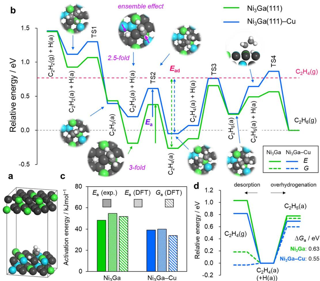
Fig. 4 DFT calculations for acetylene hydrogenation. (a) Example of the optimized structure in the slab model:  $\text{C}_2\text{H}_2(\text{a}) + \text{H}(\text{a})$  on  $\text{Ni}_3\text{Ga}(111)\text{-Cu}$ . (b) Energy landscapes of the stepwise hydrogenation from acetylene to ethane. Sum of the bare slab and gas-phase  $\text{C}_2\text{H}_6$  was set to zero in energy. (c) Comparison of activation energies. (d) Energy diagrams of ethylene desorption and overhydrogenation.
