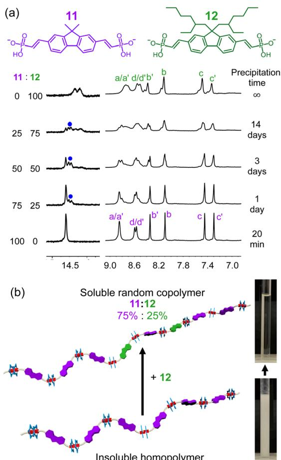
Fig. 8 (a)  $^1\text{H}$  NMR spectra of homopolymers and copolymers involving **11** and **12** (5 mM cyanostar, 298 K, 600 MHz,  $\text{CD}_2\text{Cl}_2$ ). (b) Pictures of solutions and representations of the homopolymer formed with monomer **11** and a copolymer of monomer **11** and **12**.
