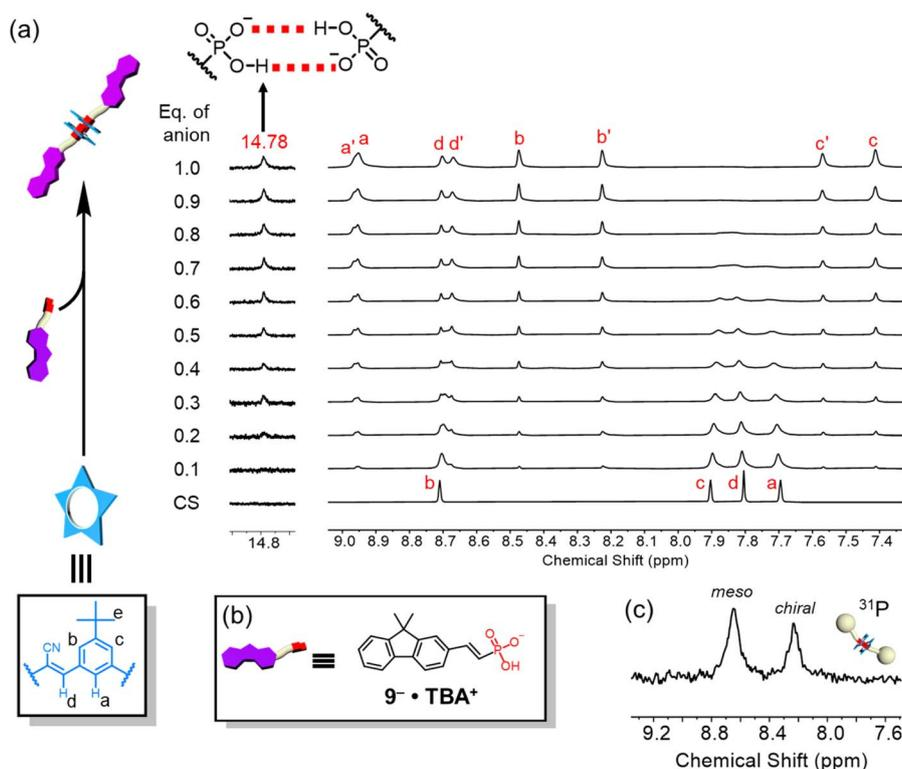
Fig. 2 (a) Titration of dimethyl fluorene vinyl phosphonate **9** into cyanostar (1 mM, CD<sub>2</sub>Cl<sub>2</sub>, 298 K, 600 MHz). (b) Structure of tetrabutylammonium salt of dimethyl fluorene vinyl phosphonate. (c) <sup>31</sup>P NMR spectrum at equivalence point (1 mM, CD<sub>2</sub>Cl<sub>2</sub>, 298 K, 202 MHz).
