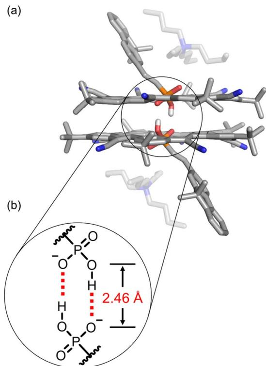
Fig. 3 (a) Crystal structure of 2 : 2 cyanostar : phosphonate complex with **9** with the presence of two tetrabutylammonium cations. (b) The pair of self-complementary hydrogen bonds are observed at a O...O distance of 2.46 Å. Data collected at 150 K. Non-polar hydrogen atoms and disorder of cyanostar and phosphonate omitted for clarity (CCDC 2263985).
