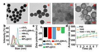
Fig. 2 (a) TEM images of (i)  $sSiO_2$ , (ii)  $sSiO_2@MnO_2$ , (iii)  $HMnO_2$  and (iv) MPL. Scale bar: 100 nm. (b) The size distribution of different nanoparticles. (c) The zeta potential of different nanoparticles. (d) The stability of MPL@ICC within 7 days when stored in different solutions.
