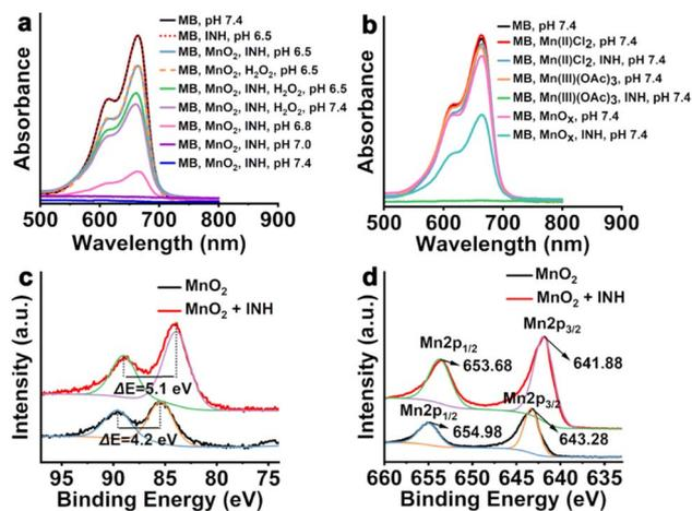
Fig. 1 (a) (b) UV-vis absorption spectra of MB after degradation in different solutions. (c) Mn 3s and (d) Mn 2p spectra of MnO<sub>2</sub> and MnO<sub>2</sub> + INH. MB: methylene blue; INH: isoniazid.
