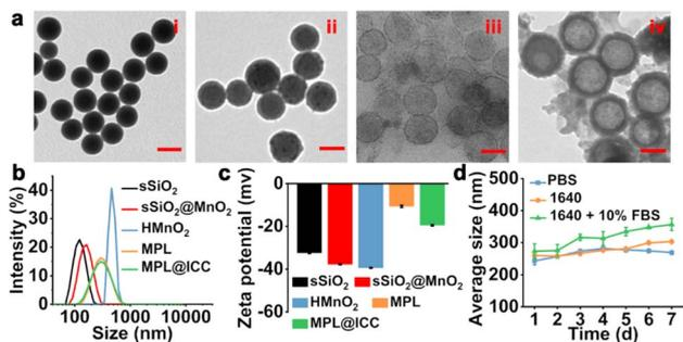
Fig. 2 (a) TEM images of (i) sSiO<sub>2</sub>, (ii) sSiO<sub>2</sub>@MnO<sub>2</sub>, (iii) HMnO<sub>2</sub> and (iv) MPL. Scale bar: 100 nm. (b) The size distribution of different nanoparticles. (c) The zeta potential of different nanoparticles. (d) The stability of MPL@ICC within 7 days when stored in different solutions.
