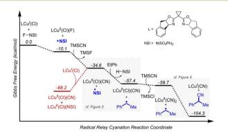
Fig. 2 Full reaction thermodynamics for Cu/NFSI-catalysed benzylic cyanation. Gibbs free energies (kcal  $mol^{-1}$ ) are computed at M06-D3(0)/basis-II/SMD(CH<sub>2</sub>Cl<sub>2</sub>)//M06-D3(0)/basis-I level of theory.
