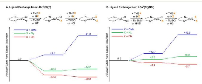
Fig. 5 Ligand exchange thermodynamics starting from two key  $Cu^{II}$  resting states: (A)  $LCu^{II}(CI)(F)$  and (B)  $LCu^{II}(CI)(NSI)$ . L = bis(oxazoline) ligand shown in Fig. 2. Gibbs free energies (kcal  $mol^{-1}$ ) are computed at 298.15 K at the M06-D3(0)/basis-II/SMD( $CH_2CI_2$ )//M06-D3(0)/basis-I level of theory.
