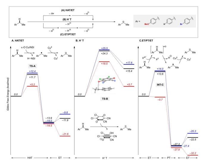
Fig. 8 Energy landscape for benzylic cation formation through (A) hydrogen-atom transfer/electron transfer (HAT/ET), (B) hydride transfer (H $^-$ T), and (C) electron/proton/electron transfer (ET/PT/ET) *via* Ir<sup>III\*</sup>. Results for three *para* substituted benzylic substrates are shown in blue (p-Br), black (p-H) and red (p-OMe). Gibbs free energies are in kcal mol $^{-1}$  computed at 298.15 K at the M06-D3(0)/basis-II/SMD(CH $_2$ Cl $_2$ )//M06-D3(0)/basis-I level of theory.
