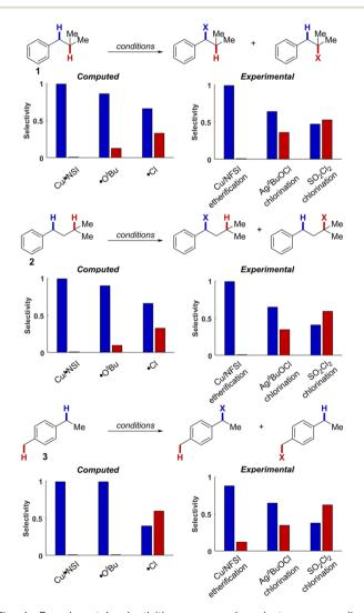
Fig. 4 Experimental selectivities compared against corresponding computational values derived from Gibbs free energies computed at 298.15 K at the M06-D3(0)/basis-II/SMD(CH $_2$ Cl $_2$ )//M06-D3(0)/basis-I level of theory.
