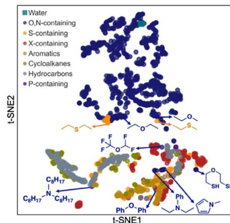
Fig. 7 2D plot of t-distributed stochastic neighbor embeddings (t-SNEs) for the latent vectors of 1447 solvents obtained from Student 35 model.
