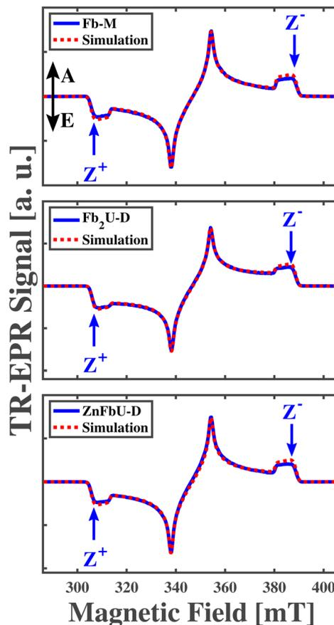
Fig. 5 Spin-polarized triplet cw time-resolved EPR spectra of Fb-M (top panel), Fb<sub>2</sub>U-D (middle panel), and ZnFbU-D (bottom panel) measured at 20 K. Arrows in each panel indicate magnetic field positions in the EPR spectra at which ENDOR experiments have been performed. The directions of absorptive and emissive transitions are shown as vertical arrows labeled as A and E, respectively, in the top panel.
