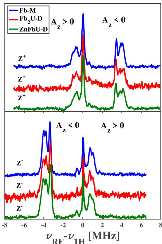
**Fig. 6** Time-resolved Mims-type ENDOR spectra of Fb-M (blue), Fb<sub>2</sub>U-D (red), and ZnFbU-D (green) measured at the  $Z^+$  (top panel) and  $Z^-$  (bottom panel) canonical fields at 20 K. Spectral regions characterized by different signs of the  $z$ -component of the hyperfine coupling tensor,  $A_z$ , are indicated in each panel.
