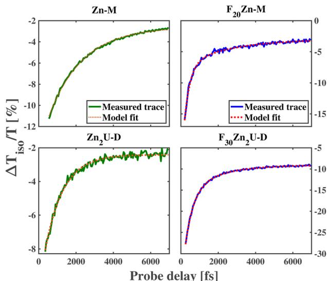
**Fig. 3** Comparisons between measured (solid) and modelled (dashed) ultrafast kinetics of the excited state absorption measured near 1.9 eV of Zn-M (top left), F<sub>20</sub>Zn-M (top right), Zn<sub>2</sub>U-D (bottom left) and F<sub>30</sub>Zn<sub>2</sub>U-D (bottom right) following photoexcitation of these molecules' B states with 2.85 eV (435 nm) pump pulses.
