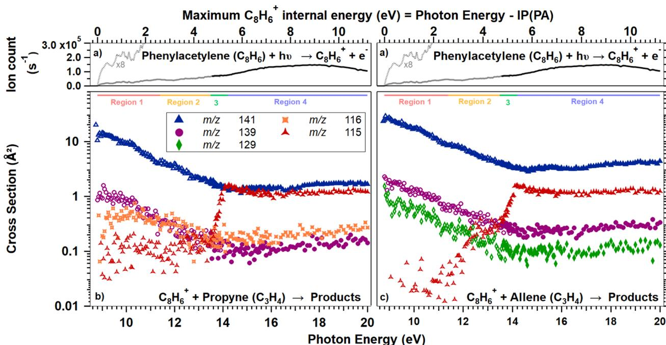
Fig. 1 The top panels (black traces) display the  $C_8H_6^+$  photoion yield starting from phenylacetylene precursor (gray region was recorded with Kr in gas filter while dark region was recorded with Ne in gas filter). Bottom panels are reaction cross sections for the products resulting from  $C_8H_6^+$  produced from phenylacetylene reacting, with (left) **propyne** and (right) **allene** as a function of photon energy.
