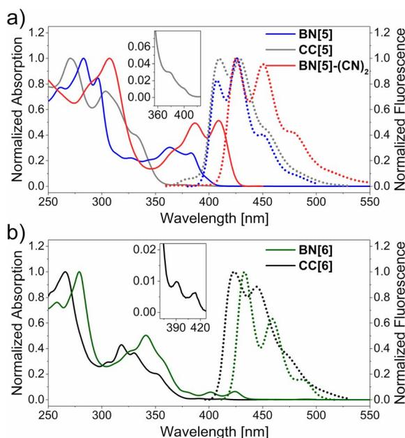
**Fig. 3** Normalized absorption (continuous lines) and fluorescence (dotted lines) spectra of pentahelicenes (a) and hexahelicenes (b) in DCM ( $c = 2.4 \times 10^{-5}$  to  $4.0 \times 10^{-5}$  M). Insets show the lowest-energy absorption (shoulder) bands of the carbohelicenes.
