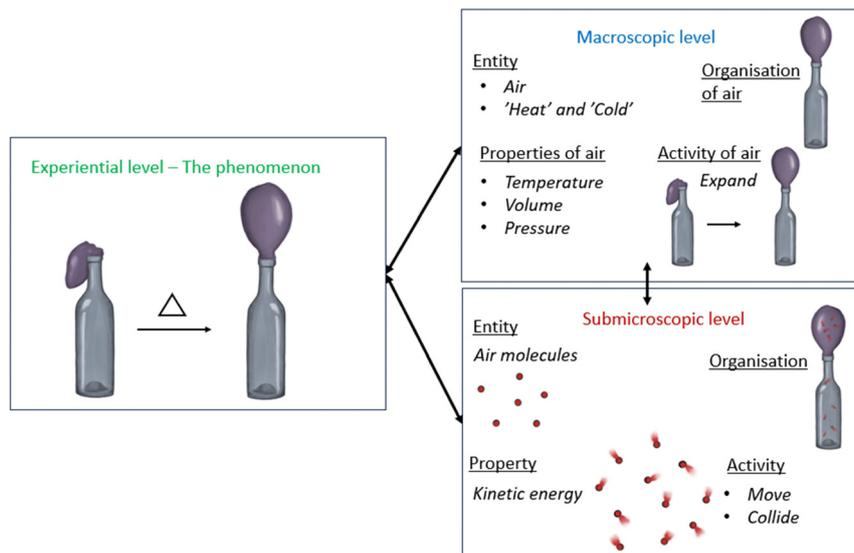
Fig. 4 Example of aspects of mechanistic features for the phenomenon of thermal air expansion in an enclosed container made up of a glass bottle and a balloon.
