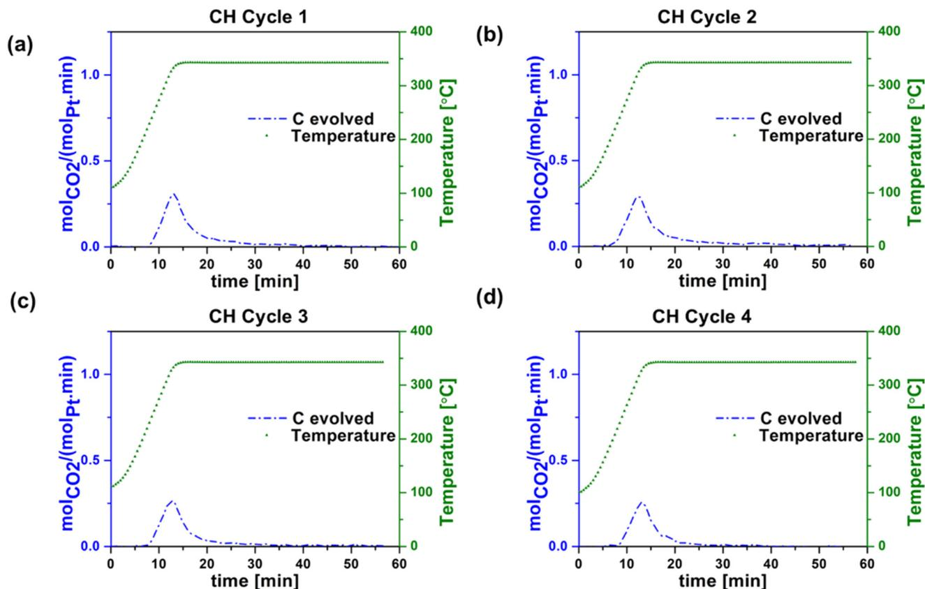
Fig. 5 Carbon evolved during regeneration step during conventional (oven) heating (CH) in (a) cycle 1, (b) cycle 2, (c) cycle 3, and (d) cycle 4. Experimental conditions: 30 sccm (20 O<sub>2</sub> in argon).
