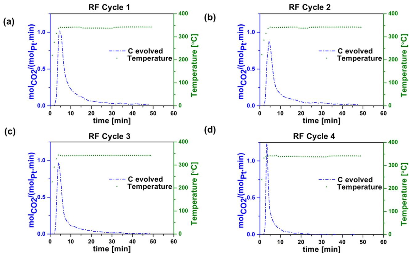
Fig. 6 Carbon evolved during regeneration step during RF heating in (a) cycle 1, (b) cycle 2, (c) cycle 3, and (d) cycle 4. Experimental conditions: 30 sccm (20% O<sub>2</sub> in argon).
