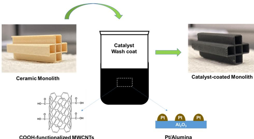
**Fig. 1** Schematic of the preparation of the catalyst used for PDH reaction: ceramic monolith is dipped in the catalyst wash coat containing MWCNT-COOH, Pt, and alumina to obtain catalyst-coated monolith.
