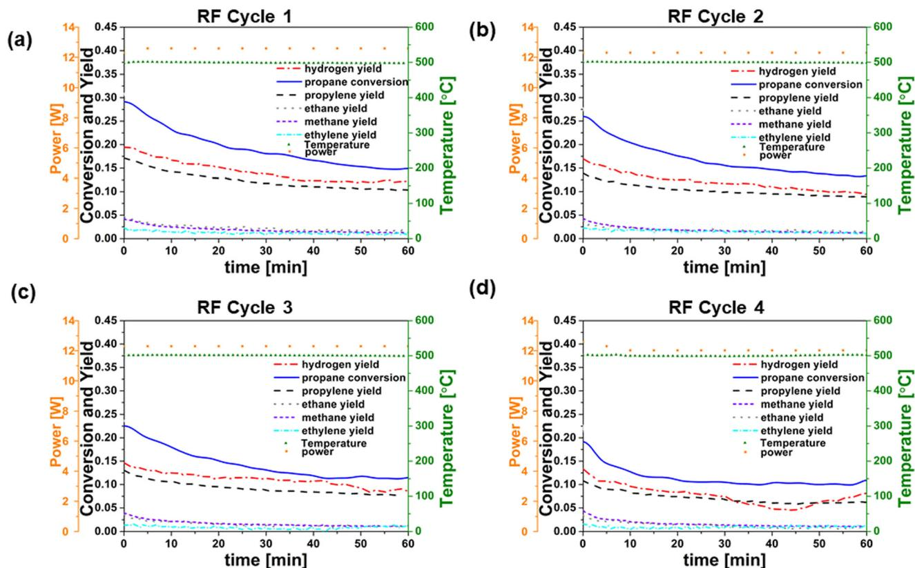
Fig. 4 Time-on-stream conversion and yield for propane dehydrogenation reaction in a washcoated monolith reactor during RF heating for (a) cycle 1, (b) cycle 2, (c) cycle 3, and (d) cycle 4. The radio frequency during each reaction cycle was chosen to be 166 MHz. Experimental conditions: 6%  $C_3H_8$ , 3%  $H_2$ , balance Ar, total flowrate = 75 sccm.
